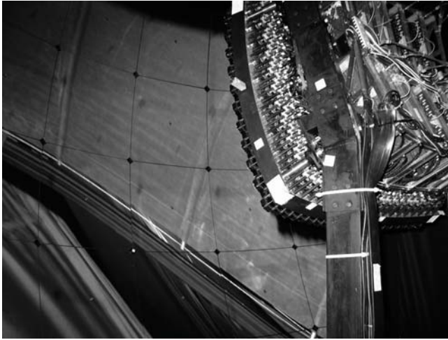
Fig. 7. Camera, consisting of 20 \times 22 photomultipliers, is facing its diamond-cut mirror
