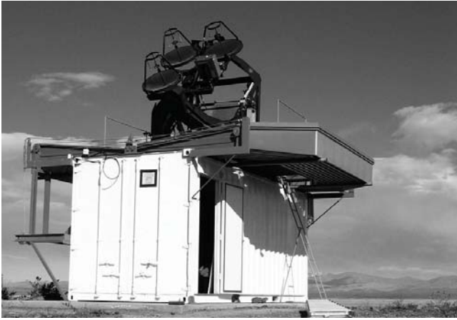
Fig. 9. On the roof of the container near the Los Leones fluorescence detector, a steerable telescope of the lidar system can be seen
