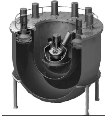
Fig. 2. Computer view of the ZEPLIN I set-up showing the target vessel with three PMTs encased in an active veto system
