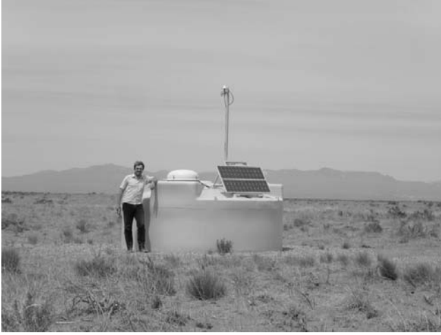
Fig. 3. One of the many water-Cherenkov detectors deployed to the Pampa Amarilla (semi-)desert. Tanks are filled with more than 10 tons of purified and deionized water. Electronics, radio, GPS, and photomultiplier tubes all run on the independent source of electric power from solar panel, stored in a battery
