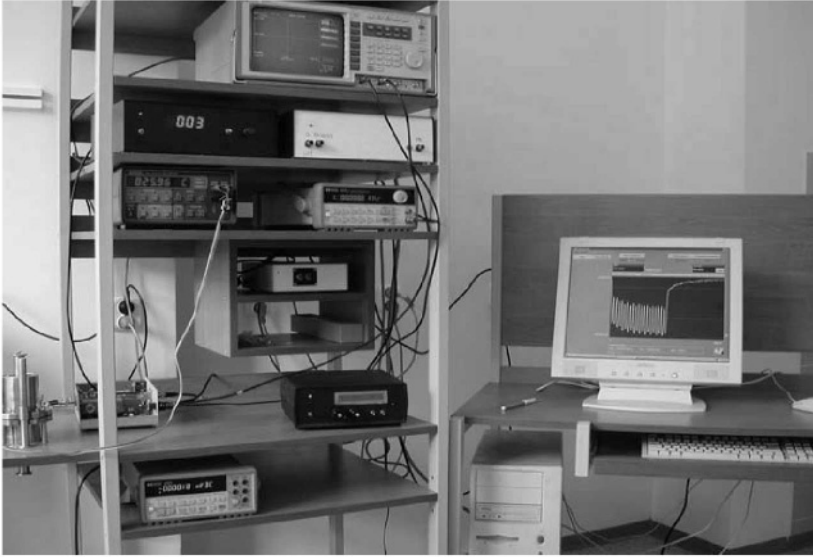
Figure 6. The dual-field, single generator MDA based NDE apparatus in the Katowice lab. At the top the MDA analyzer is placed, below they are HV AC/DC pulse unit ( U_{HV} = 20V - 1500V , \Delta t_D = 100\mu s - 1000s ) and the HV amplifier ( U_{peak-peak} < 1000V , \Delta t_D \rightarrow arbitrary and f_{HV} = DC \rightarrow 4kHz ). Below they are multimeter Keitley 195A for temperature measurement and the sine-wave frequency generator HP. At the main table they are the temperature stabilization unit (left side). Next they are the NDE measurement generator and the controller). The screen present the user-friendly software and the response of the isotropic 5CB sample to the action of a sine-wave train of a strong electric field.
