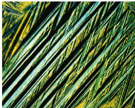
Fig. 3.11. Optical micrograph with polarized light on the surface of a Cu–Al–Zn sample after cooling through MT. Domains corresponding to different martensite variants with many different characteristic lengths coexist
