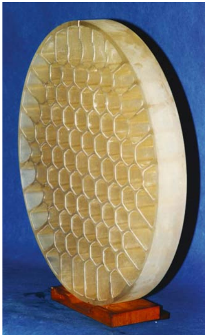
Fig. 4.51. Zerodur® lightweight mirror sample 664 mm in diameter and 72 mm in height, manufactured by direct casting by the use of a ceramic fiber mold. The weight reduction is 57% (faceplate thickness 12 mm, rib thickness 10 mm, cavity depth 60 mm, cavity width 50 mm)
