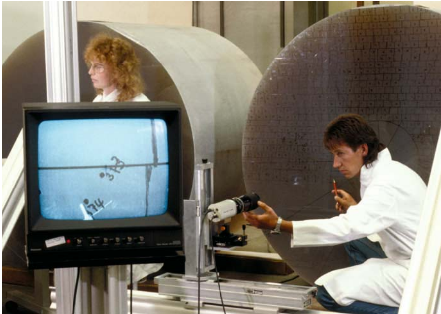
Fig. 4.55. Examining the raw castings for internal defects using an infra-red camera
