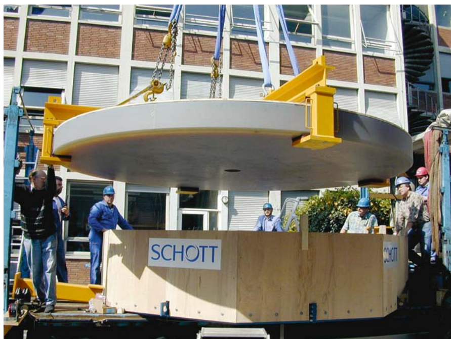
Fig. 4.77. Zerodur disk for the Wettzell Fundamental Research Station
