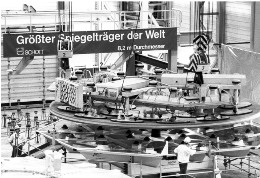
Fig. 4.39. Vacuum lifting device during delivery of the first 8.2-m Zerodur® blank of 23 t
