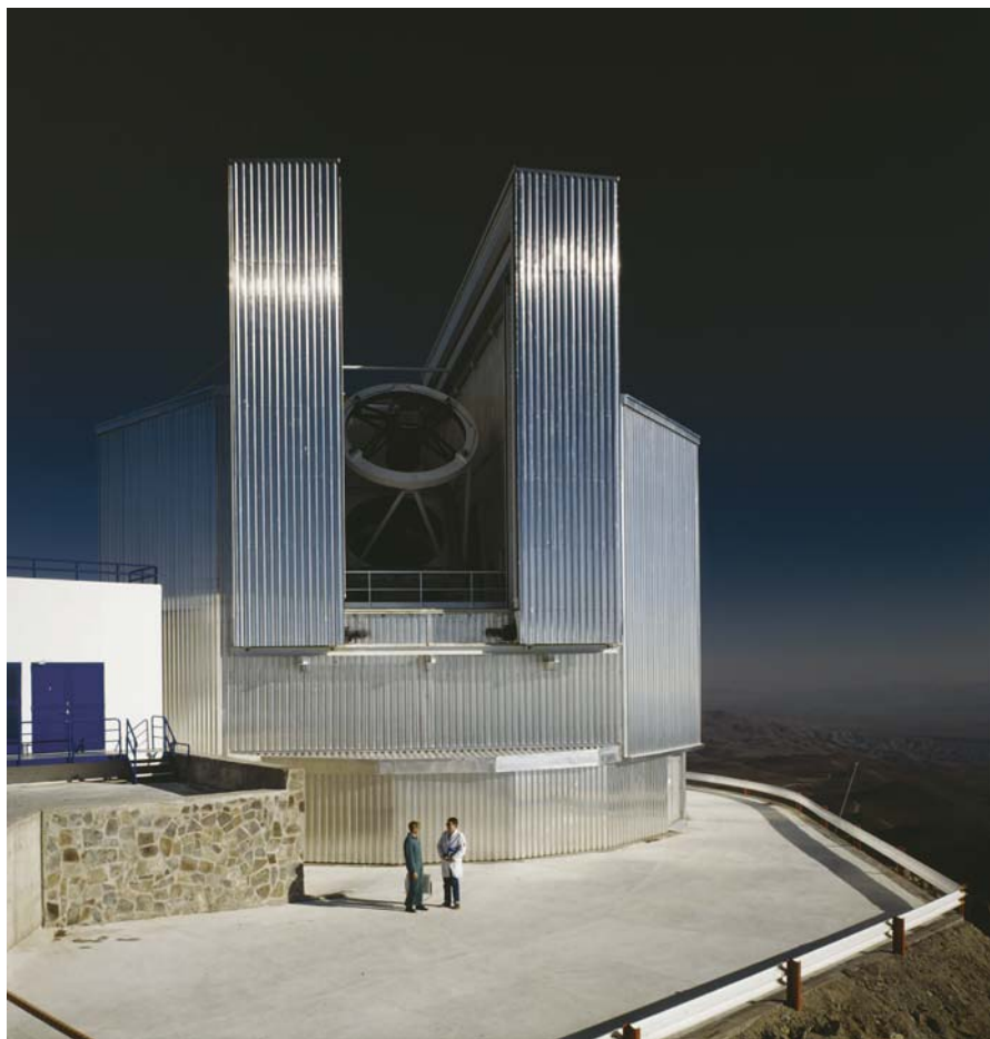
Fig. 4.67. ESO's New Technology Telescope (3.5-m Zerodur® mirror) obtains the highest performance by using active and adaptive optics
