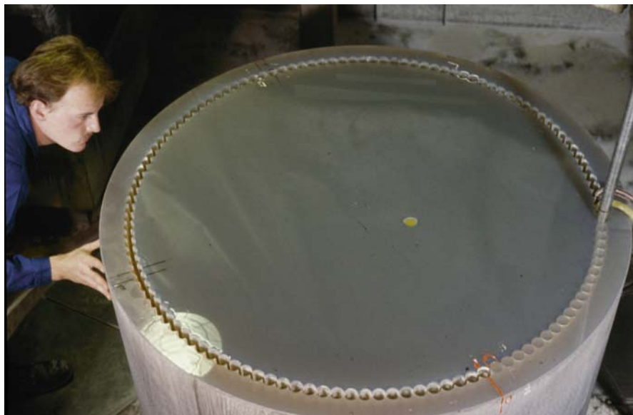
Fig. 4.56. Boring out the hollow cylinder with diamond tools
