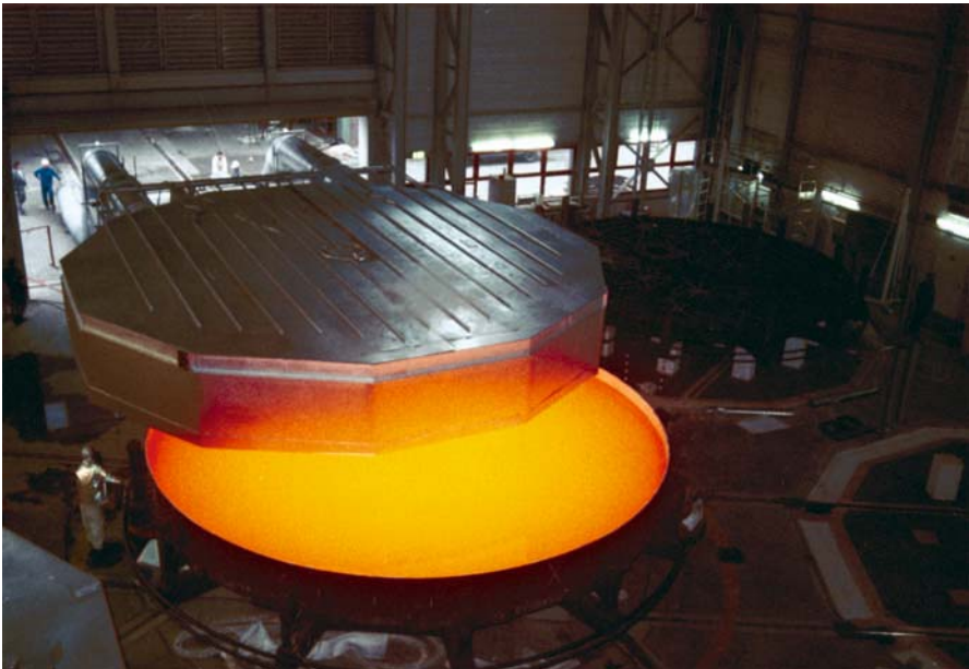
Fig. 4.28. Mold with molten glass on the centrifuge with cooling cover
