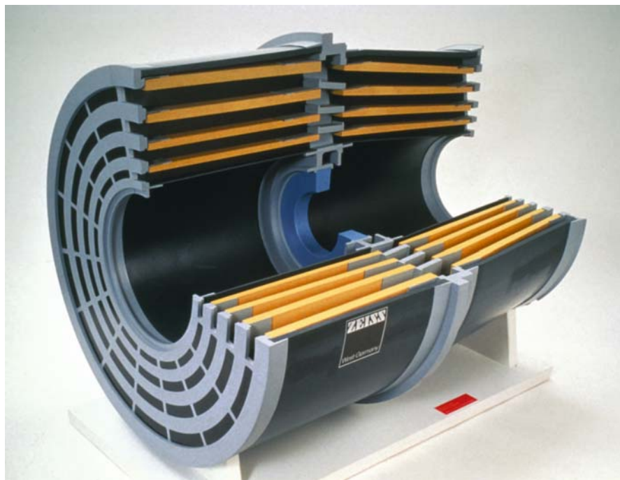
Fig. 4.71. Four parabolic and hyperbolic Zerodur® cylinders are nested into one another for the German spaceborne X-ray telescope ROSAT
