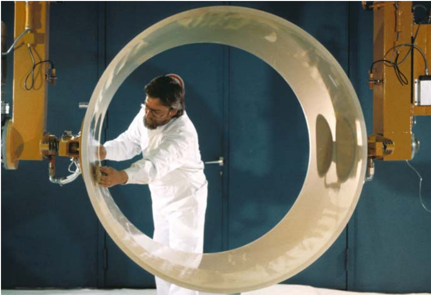
Fig. 4.72. One of twelve thin-walled conical Zerodur® cylinders of diameters up to 1274 mm for the AXAF X-ray telescope at NASA
