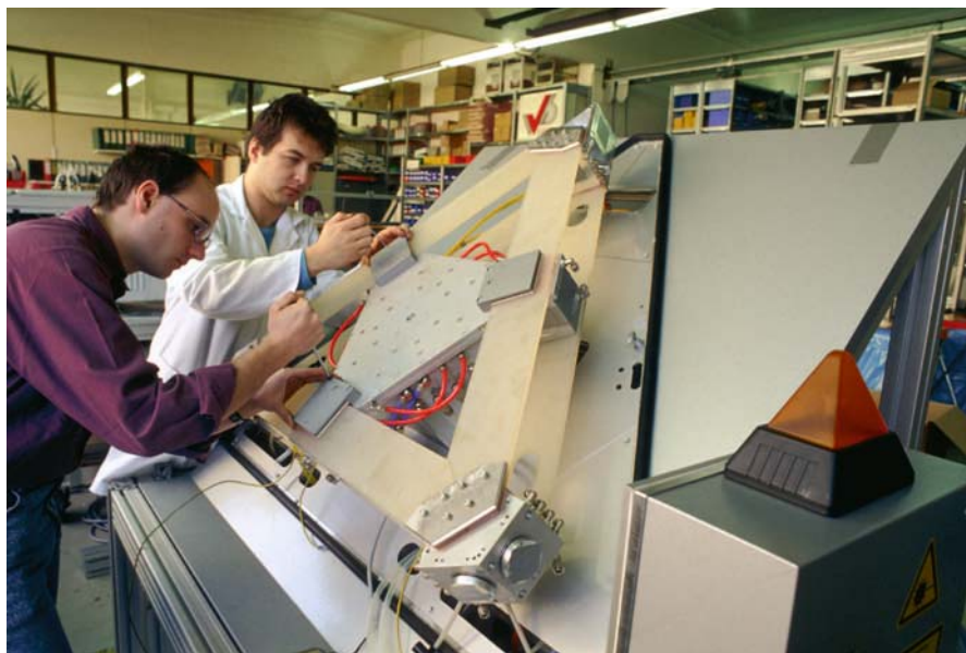
Fig. 4.78. In high-energy lasers, Zerodur® distance spacers keep the optical elements in exact position to improve the long-term stability of the focal point of the laser beam
