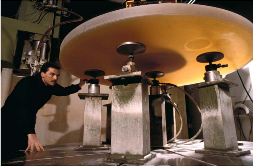
Fig. 4.68. One of 36 blanks made of Zerodur® for the 10-m Keck Telescope
