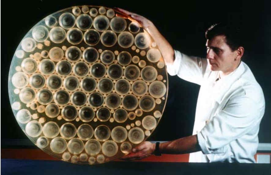
Fig. 4.70. A lightweight mirror blank made by the R.E.O.S.C. Company in France, for the Earth observation satellite SPOT
