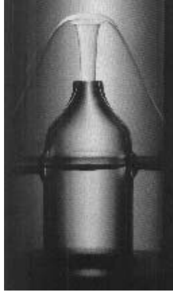
Fig. 2.7. (a) Schematic sketch of an experimental setup used to demonstrate the fountain effect. The helium inside and outside the flask has been drawn in a slightly different shade for clarity. (b) Photo of a fountain generated in helium II [47]
