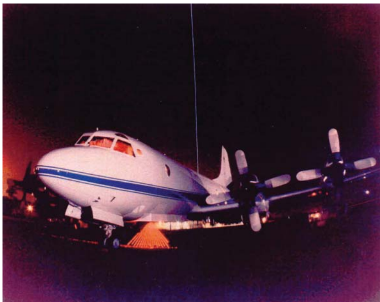
Fig. 13.19. NASA LaRC and GSFC lidars aboard the NASA P-3 for LITE validation. Downlooking beams represent a time-lapse photograph of the LASAL lidar fan beam system. The uplooking green line shows the LaRC 532 nm lidar output. (Courtesy of G.K. Schwemmer.)
