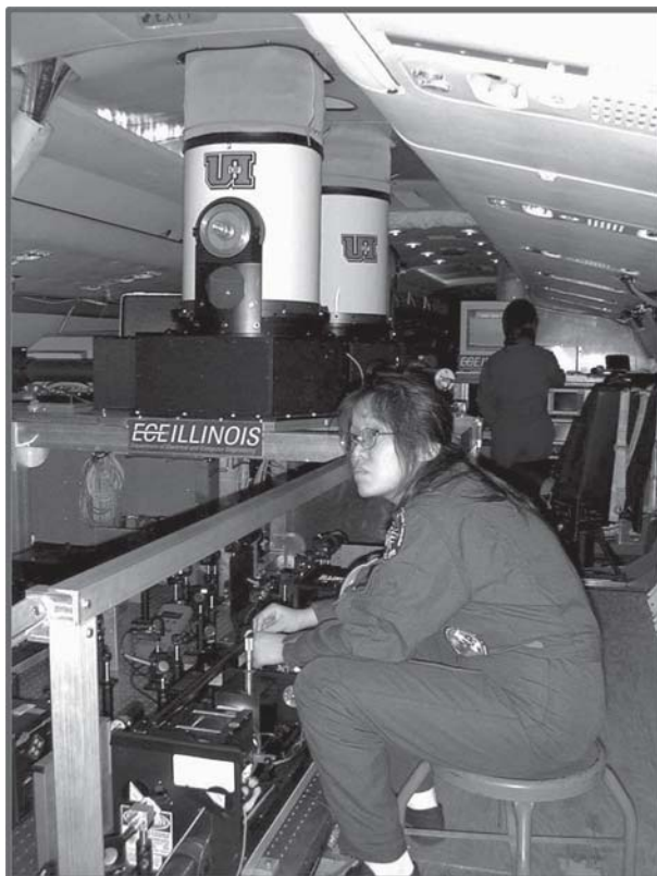
Fig. 13.3. Dr. Xinzchao Chu from the University of Illinois at Urbana-Champaign operating the Rayleigh/Fe Boltzmann temperature lidar aboard the NSF/NCAR Electra aircraft, 1991. (Courtesy of C. Gardner.)
