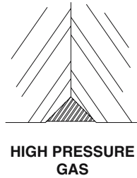
Fig. 1.4. Bridgman type gas seal applied to light-gas gun
