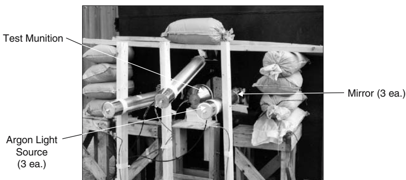
Fig. 6.16. Photo of the fragmenting liner test setup
