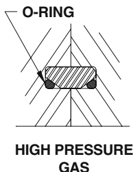
Fig. 1.5. A diamond seal that is typical of many modern light-gas gun seals
