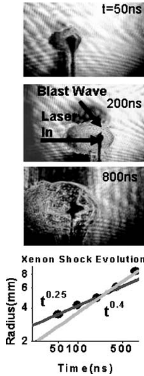
Figure 3. Images of blast waves in xenon at 50 ns, 200 ns, and 800 ns after a 1000-J drive beam has hit a 0.5-mm nylon target. The bottom panel is a graph of the radius of the blast waves as a function of time. It shows that the blast waves follow a trajectory slower than t^{0.4} before \sim 400 ns, indicating significant energy losses due to radiation.
