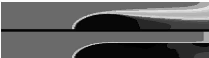
Figure 2. Radiative temperature in the shadow test with fixed eigenvalues (upper panel) or calculated ones (lower).
