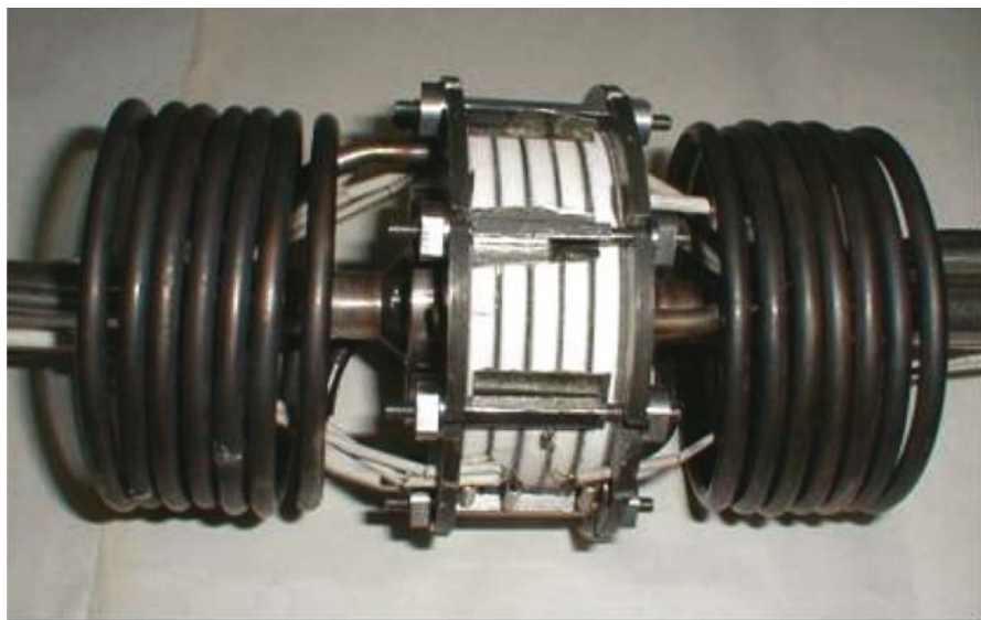
Figure 8. 5-cell stack of round cells with supported electrolyte before a test.
