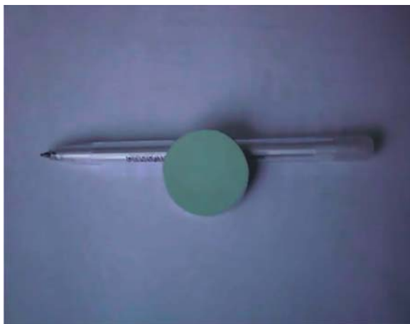
Figure 2. Three-layered SOFC membrane.
