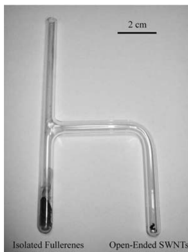
Fig. 5.1. Fullerenes and open-ended SWNTs in a glass ampoule. Prior to the doping, the SWNTs and the fullerenes were degassed at \sim 200^\circ\text{C} in a vacuum. High-yield nano-peapods are produced after heating for several days at 400\text{--}500^\circ\text{C}
