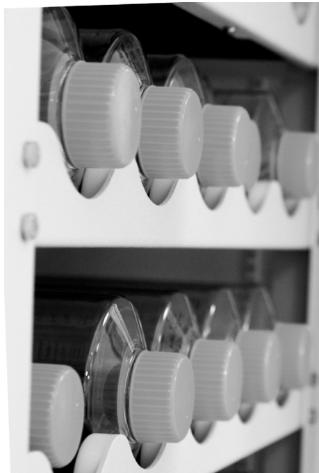
Figure 10.1 Scale-up of roller bottle culture is achieved by increasing the number of roller bottles (Photograph courtesy of Eden Biodesign).
