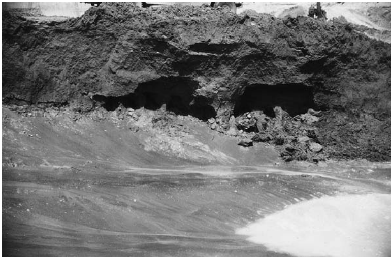
Figure 4.12 Spring sapping. Local spring sapping has caused the two cavities at the center of the photograph with outwash fans of almost liquid sand in the foreground.
