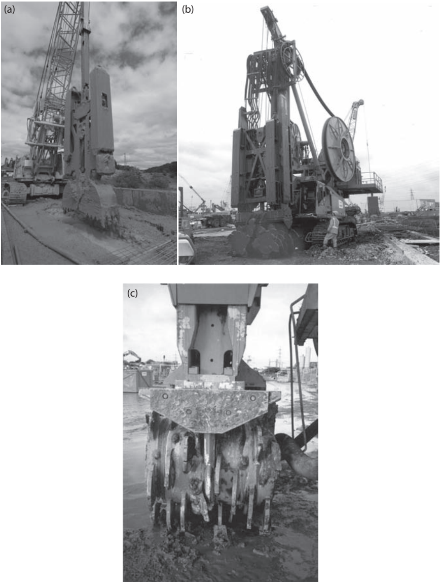
Figure 12.12 Excavation equipment for diaphragm walls. (a) Diaphragm walling grab. (Courtesy of Bachy Soletanche, Burscough, U.K.) (b) Hydromill diaphragm walling rig. (Courtesy of Cementation Skanska Foundations, Maple Cross, U.K.) (c) Close-up of rotating cutters on hydromill. (Courtesy of Cementation Skanska Foundations, Maple Cross, U.K.)
