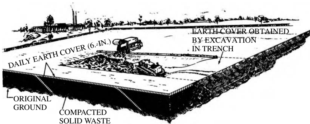
FIGURE 14 Trench method. The waste collection truck deposits its load into the trench where the bulldozer spreads and compacts it. At the end of the day the dragline excavates soil from the future trench; this soil is used as the daily cover material. Trenches can also be excavated with a front-end loader, bulldozer, or scraper. From Sanitary Landfill Factors , Thomas J. Sorg and H. Lanier Hickman, U.S. Department of Health, Education and Welfare, Public Health Service Publication N. 1792, Superintendent of Documents, Washington, DC, 1970.
