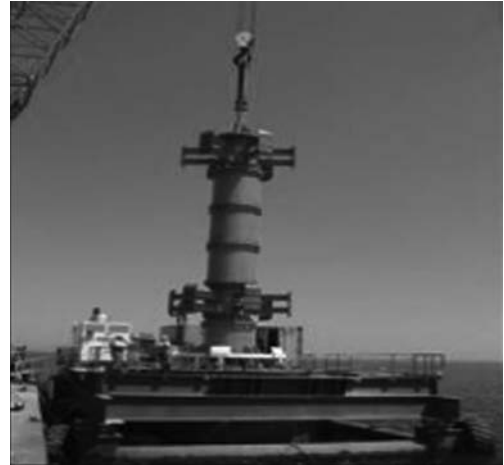
Figure 3. Wirth RCD drill used on Oak Creek project, Chicago, Illinois.
