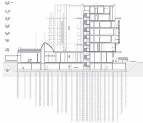
Figure 6. Section A' of building A/B/C, with Discrepile.
