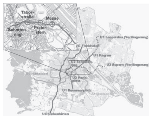
Figure 6. Site plan of U2 line extension, circles show stations equipped with geothermal energy plants.
