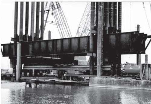
Figure 19. Static axial load test set up.
