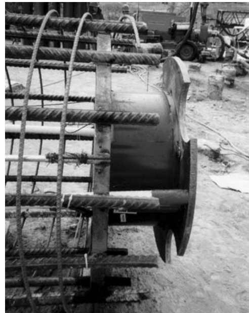
Figure 21. Osterberg load cell.
