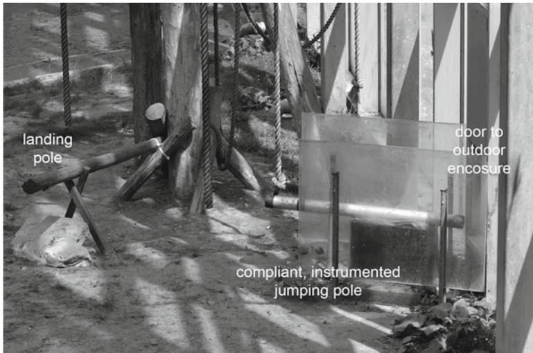
**Fig. 3.2** Setup for studying jumping in gibbons. The setup consists of an aluminium pole with adjustable compliance, mounted onto a force plate. In addition (not visible), two high-speed video cameras are installed (for a full description of the setup see Channon et al. 2010 and in press)
