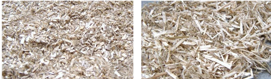
Fig. 1: Technical hemp: on the left, hemp shives fraction A; on the right, hemp shives fraction B
