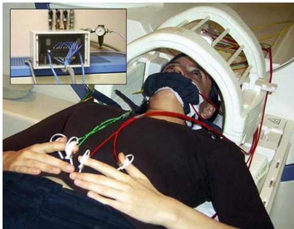
Fig. 4.5. Fully automated pneumatically driven tactile stimulation. Flexible membranes (4D Neuroimaging, Aachen, Germany) connected to pressure resistant pneumatic tubes transmit the stimuli to the lips, fingers or toes (not shown). Upper left: the 24-channel high precision electromagnetic valve system was designed to investigate somatosensory somatotopy (Reprinted from Radiologie up2date 4/2005 317–336 with permission)
