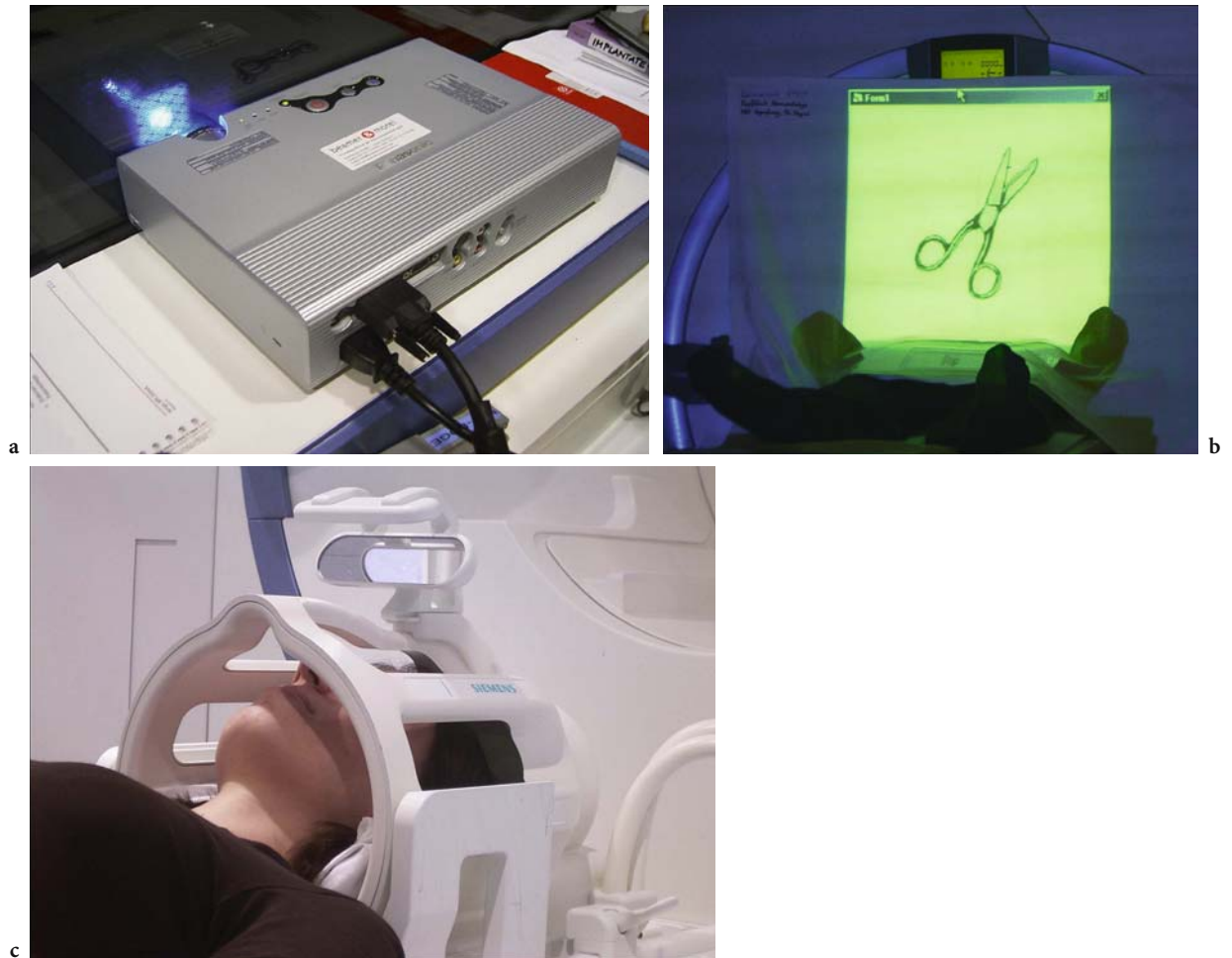
Fig. 4.4a-c. Typical equipment for visual stimulation. a High resolution video beamer. As for all electronic devices, a placement outside the scanner room should be preferred to avoid imaging artifacts. b Semitransparent projection screen mounted to the scanner bore. c Commercial mirror system for back-projection mounted to the head-coil (Reprinted from Radiologie up2date 4/2005 317–336 with permission)
