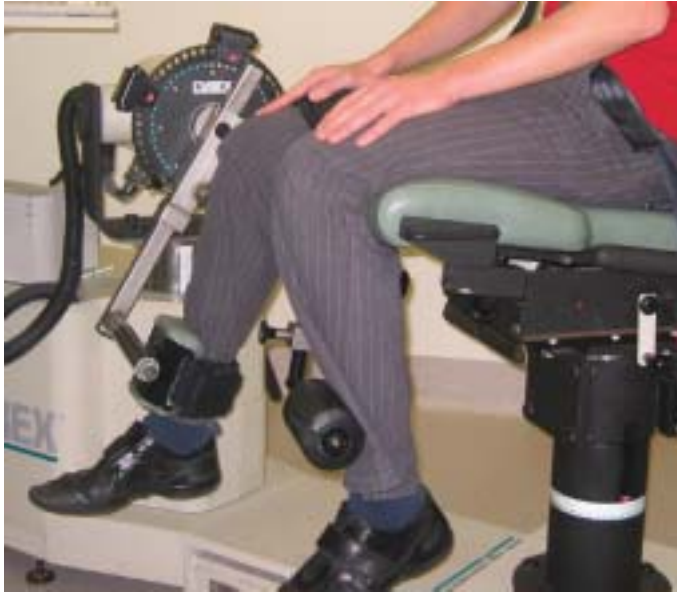
Fig. 5. – Computerised device for assessment of isometric and isokinetic muscle strength.
