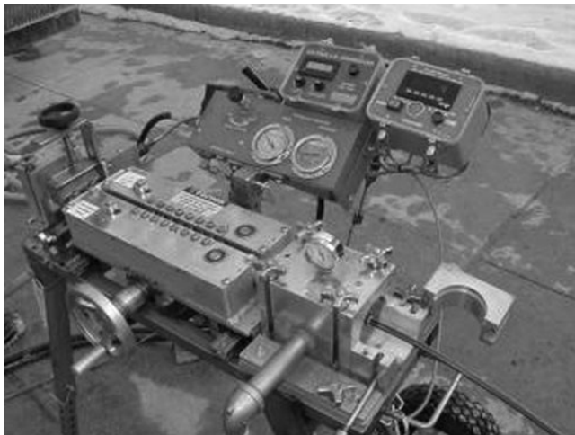
Figure 4-8. Commercially Available Low Air-Speed Blown-Cable Equipment, Including an Integral Cable Pusher (Courtesy of A-D Technologies).
