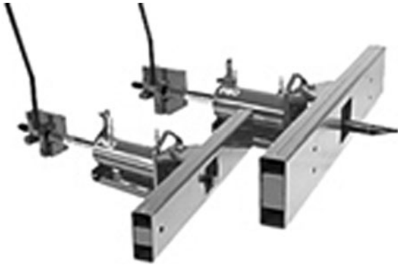
Figure 3-13. Rod Pusher (Courtesy of Ditch Witch).
