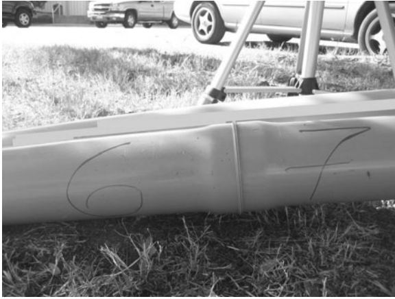
Figure 6-3. Field-Fused PVC Joint.
