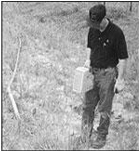
Figure 3-15. A Walkover Locator Used with a Steerable Piercing Tool (Courtesy of TT Technologies).
