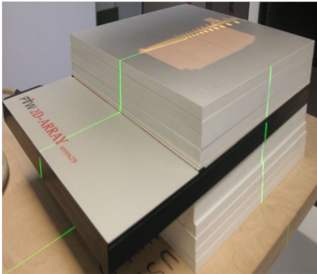
Fig. 20.3 Combination of array and phantom
