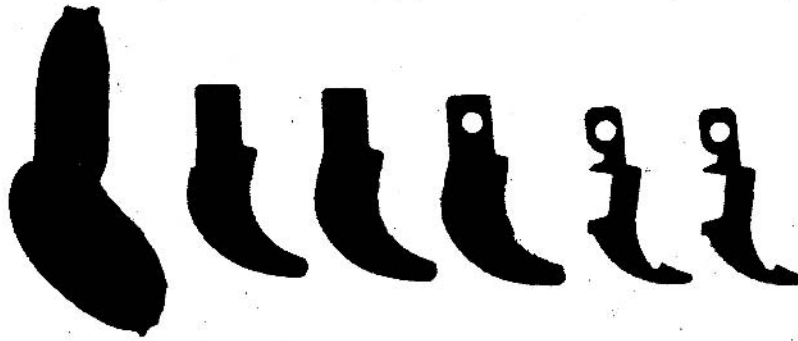
Fig. 6.2 Sequence of machining operations for M1 safety [3, p 121]
