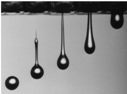
Figure 4.12 Formation of a liquid droplet at the dip of a piezoelectric dispenser. The figure was kindly provided by Microdrop Gesellschaft für Mikrodosiersysteme mbH (Norderstedt, Germany).
