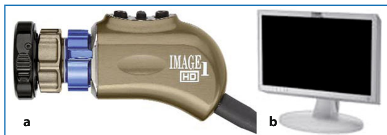
Fig. 1.3 High-definition (HD) cameras a offer the ultimate image quality. They require a full HD 16:9 flat monitor b in order to visualize the HD images
