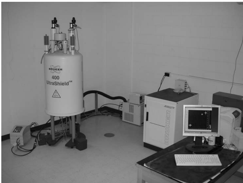
Figure 7.2 A modern NMR spectrometer showing from left to right a 400 MHz superconducting magnet, electronics console including an acquisition computer and radiofrequency amplifiers, and keyboard and monitor for the PC which inputs parameters and commands to, and extracts data from, the spectrometer
