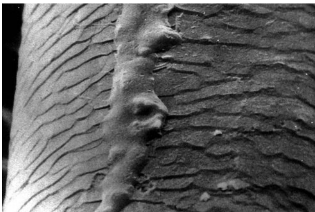
Fig. 8.3 Setting lotion deposit on hair surface
