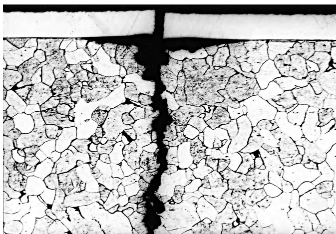
Figure 14.2. Undermining of nickel electrodeposit on steel by galvanic corrosion in 3% NaCl solution (100 \times ). Crack resulted from cyclic stressing in a corrosion-fatigue test [H. Spähn and K. Fässler, Werkst Korros. 17 , 321 (1966)].
