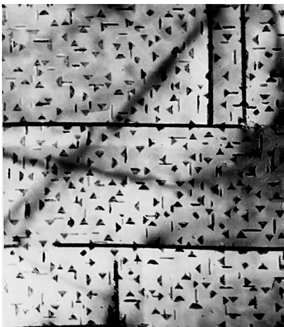
Figure 11.1. Nuclei of \text{Cu}_2\text{O} formed on copper surface at 10^{-1} mmHg oxygen pressure (13.3 Pa), 525^\circ\text{C} , 20s (17,600 \times ). Black lines are bands of imperfections (stacking faults) in the copper lattice (Brockway and Rowe [5]).
