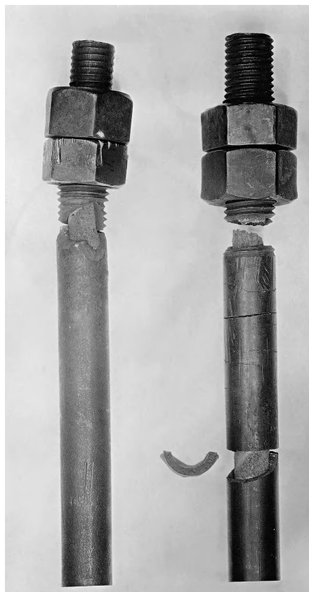
Figure 20.5. Layer-type dezincification in brass bolts (actual size).
