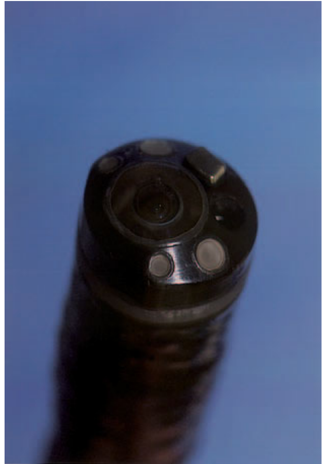
Fig. 30.11 Tip of a prototype Olympus colonoscope with variable angle of view (160–210 degrees). The convex lens protrudes from the colonoscope tip.
