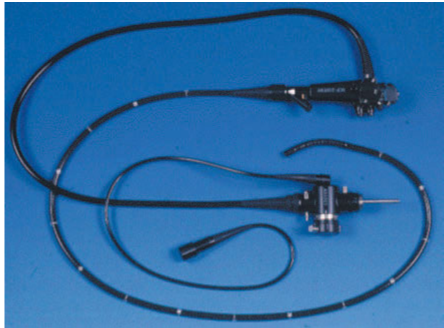
Fig. 24.14 A variable-stiffness/imager colonoscope (prototype). Note the variable-stiffness dial situated below the instrument head and the additional umbilical that contains the imager electronics.
