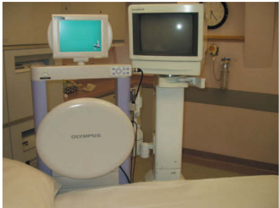
Fig. 24.5 Scope-guide system (semi-diagrammatic view) showing stand-alone unit and dedicated endoscope with in-built magnetic field generator coils.
