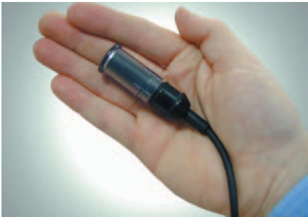
Fig. 24.10 Hand-pressure sensor with a finger grip that is easy to hold by the endoscopy assistant.
