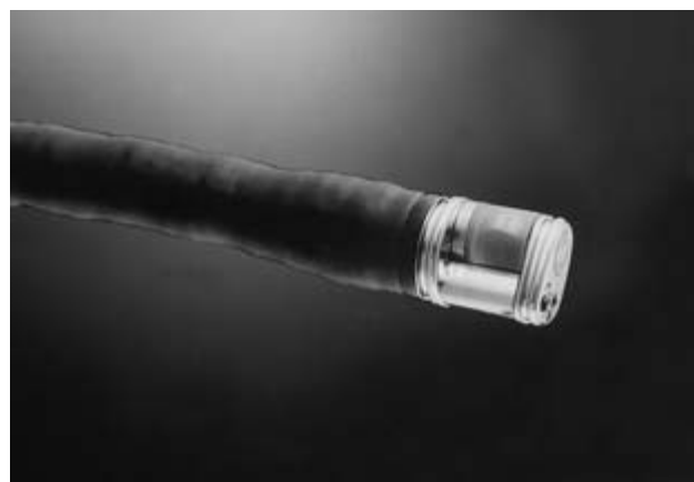
Fig. 1.31 Tip of EUS radial colonoscope (Olympus CF-UM3)—can be used with or without water balloon in place.
