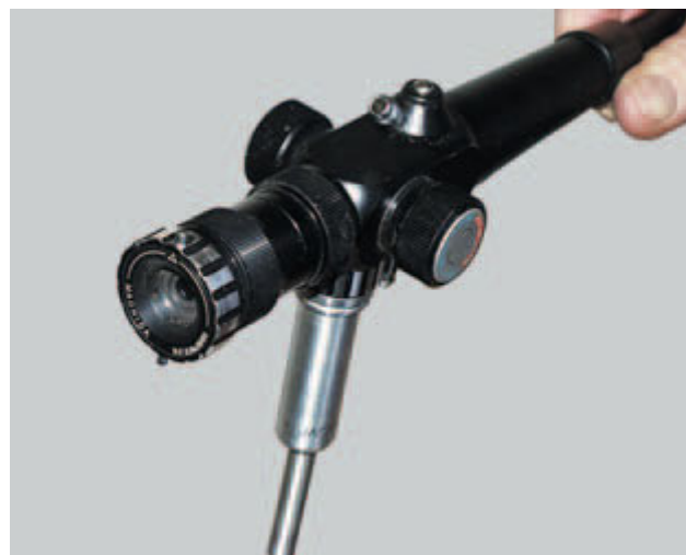
Fig. 1.22 Machida fibercolonoscope control body (1970)—note right- and left-hand controls, giving four-way tip angulation.
