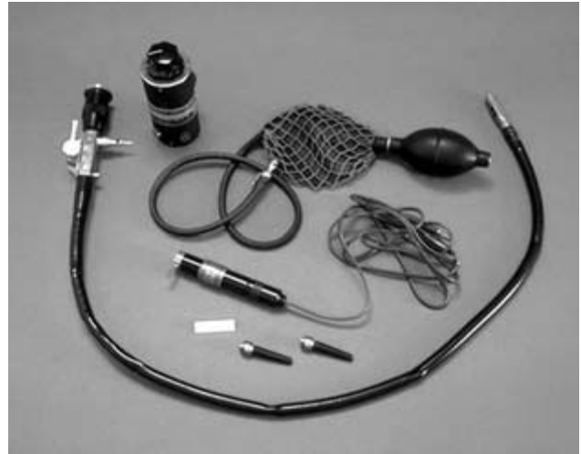
Fig. 1.15 Commercialized Hirschowitz fiberoptic gastroscope (American Cystoscope Makers Inc., ACMI, 1964), as also used in colon. Side-viewing, no angulation controls (focussing lever only), with transformer for distal tip light bulb.
