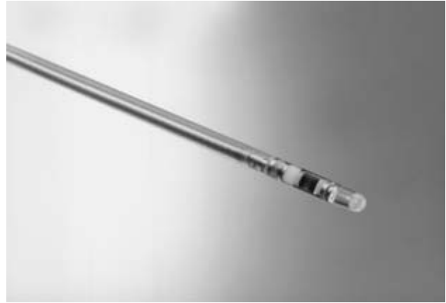
Fig. 1.33 EUS probe with motor-driven rotating transducer inside.
