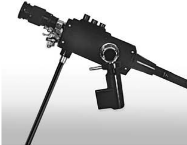
Fig. 1.16 ACMI F9A “flag-handle coloscope” (1974) with single-lever giving four-way angulation control.
