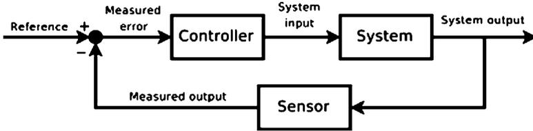
Fig. 5.12 A diagrammatic representation of a system with feedback control (Reproduced from [http://en.wikipedia.org/wiki/File:Feedback\\_loop\\_with\\_descriptions.svg](http://en.wikipedia.org/wiki/File:Feedback_loop_with_descriptions.svg))
