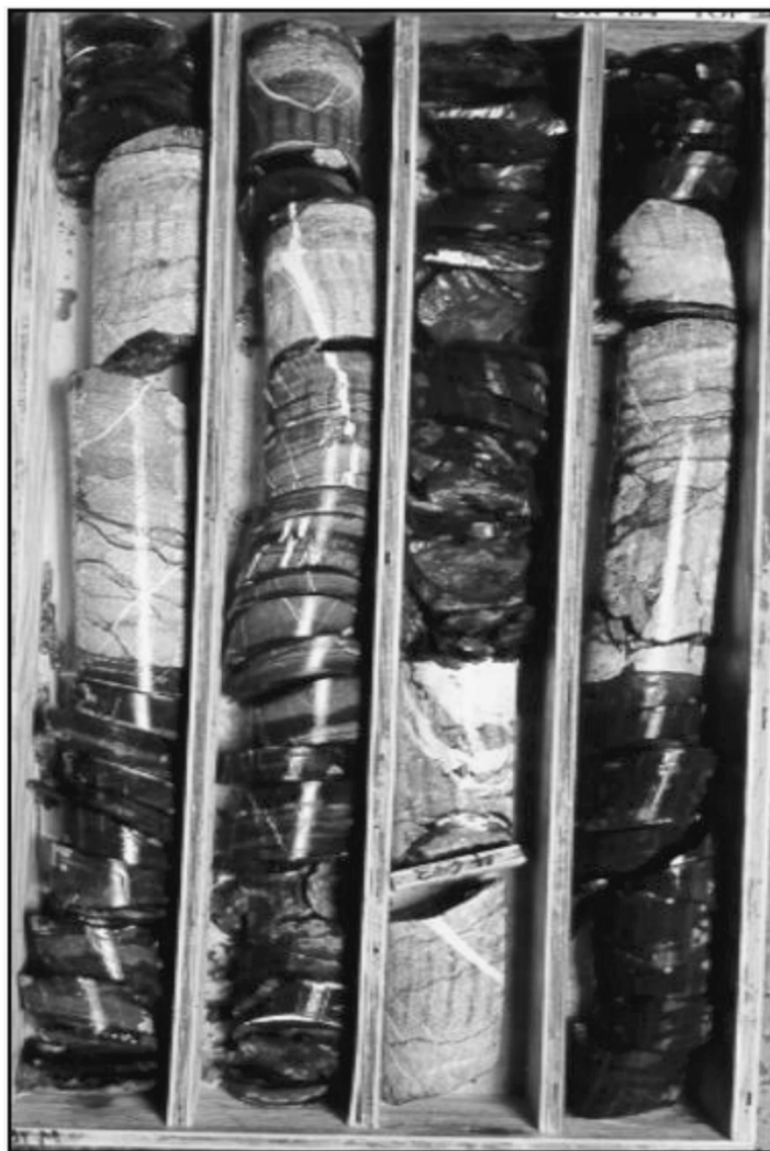
FIGURE 1.3 (See color insert) Pictorial example of bedrock core obtained near the experimental site showing the interbedded fractured shale (black) and limestone (white/gray) that dominates the saturated zone.
