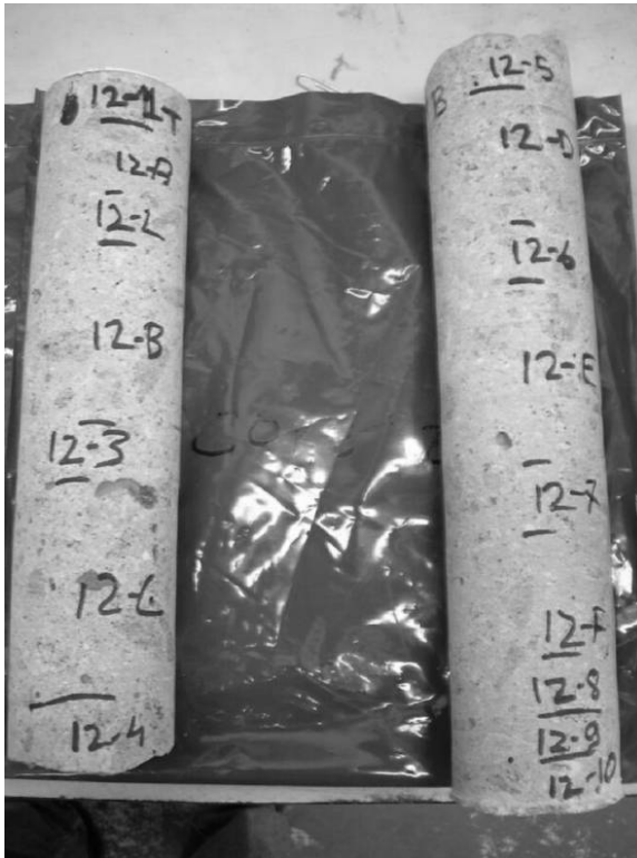
4.17 Stratification of core for determination of chloride profile.
