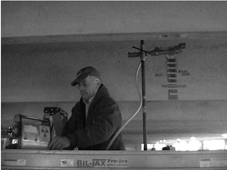
4.26 Radiographic source, collimator and lead letter template included in the frame for reference to the end of the member.
