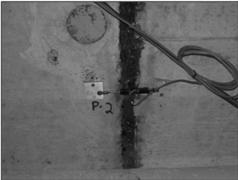
3.9 Potentiometer in use to measure the crack movement over a year. (Courtesy of WJE)
