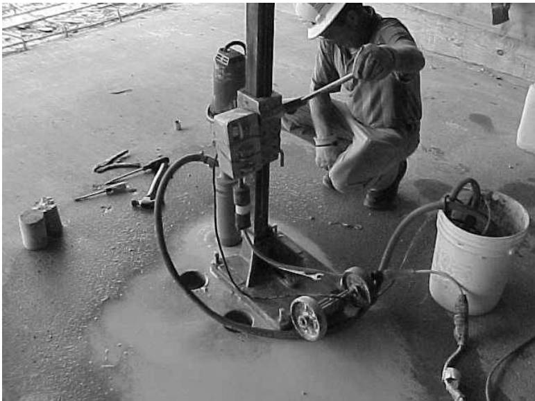
4.27 Removal of cores with an electric drill and water-cooled coring bit.
