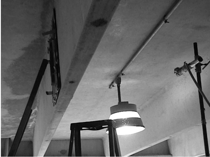
4.23 Member of interest located between radiographic film and source.
