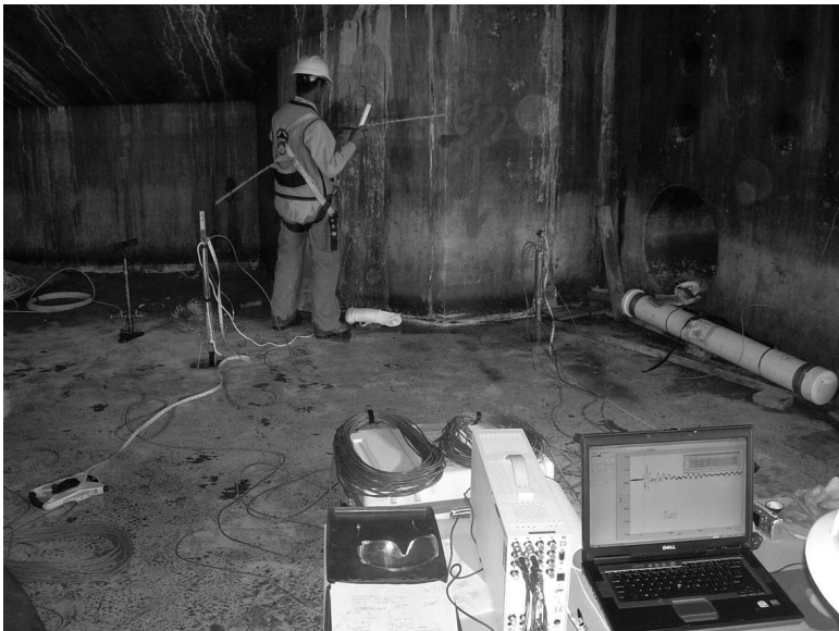
4.15 Crosshole sonic logging of an existing deep foundation.
