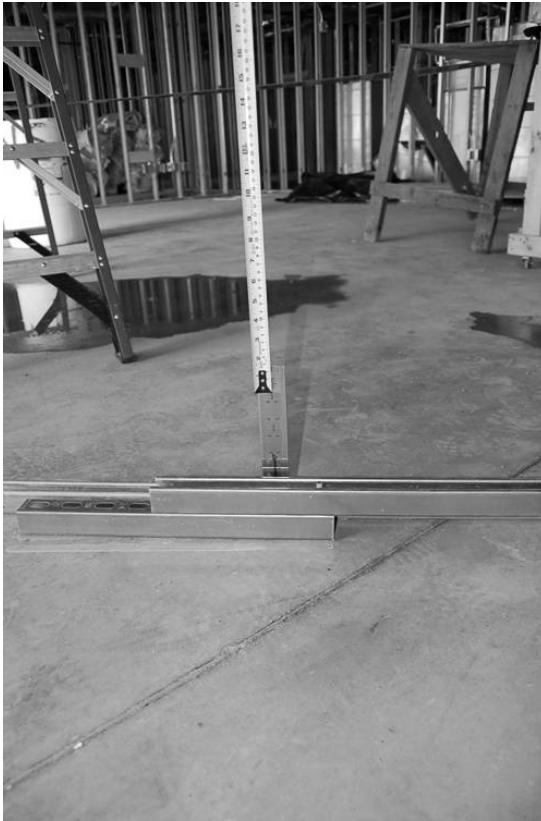
4.34 Suspended tape measure as a means of measuring deflections.
