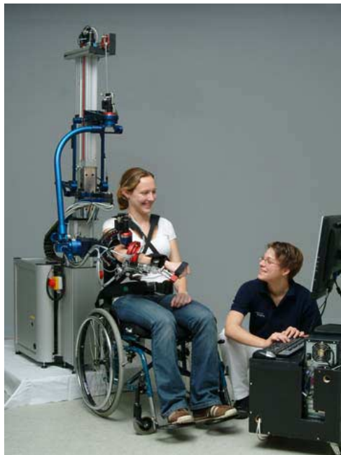
Figure 6. ARMin robot is one of the recent exoskeleton devices (ETH Zürich)
