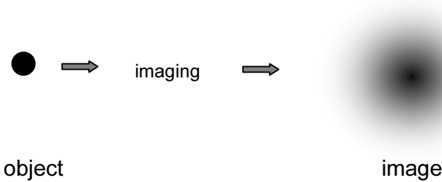
Figure 13. Principle of the point spread function (PSF)
