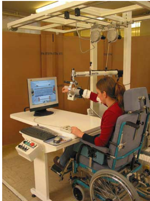
Figure 7. GENTLE/S project rehabilitation environment as an example of end effector approach
