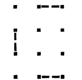
The locations of braced frames or shear walls must be considered in relation to the elevation and plan of the building.
