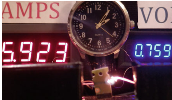
Fig. 14.50 First visible combustion occurred at elapsed time of 4 s, Power is 4.5 W. Note The power level change is not forced but is due to a decrease in resistance of the current carrying wire
