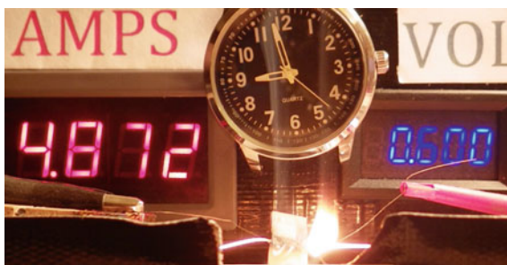
Fig. 14.37 Elapsed time from zero power is 4 min 14 s, 2.92 W. Initial flame (real time captured in video is 08:57:23)
