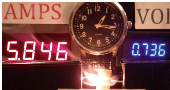
Fig. 14.23 Elapsed time from zero power is 9 s, 4.30 W. Flames burst from openings (real time captured in video is 01:16:18)
