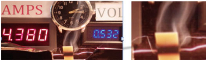
Fig. 14.5 Result of 1.8 W being applied for 1 min after the preceding 1.3 W level (elapsed time from power up is 4 min)
