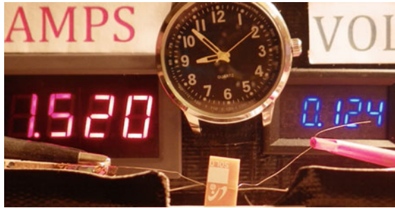
Fig. 14.32 Elapsed time from zero power ~ 1 s, 0.25 W. No visible smoke or charring (real time captured in video is 08:53:09)
