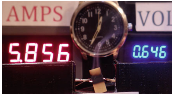
Fig. 14.12 Elapsed time from zero power is 50 s, 3.78 W. Smoke has diminished (real time captured in video is 12:35:00)
