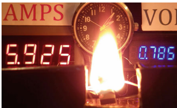
Fig. 14.47 Elapsed time from zero power is 31 s, 4.7 W. Engulfing flame (real time captured in video is 02:06:50)
