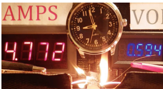
Fig. 14.38 Elapsed time from zero power ~4 min 25 s, 2.92 W. Flame continues (real time captured in video is 08:57:34)
