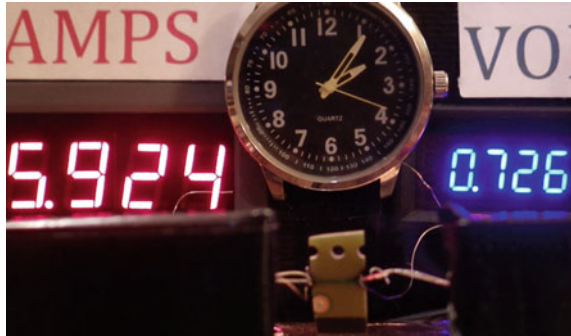
Fig. 14.49 Applied 4.3 W at 02:06:18. No visible combustion at power up
