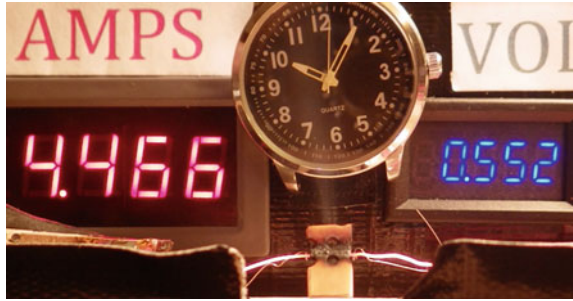
Fig. 14.61 Elapsed time from zero power is 2 min 55 s, Stepped up to 2.5 W smoke nearly gone (real time captured in video is 10:06:01)
