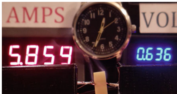
Fig. 14.10 Elapsed time from zero power \sim 1 s, 3.72 W. Wisp of smoke with no visible charring (real time captured in video is 12:34:10)
