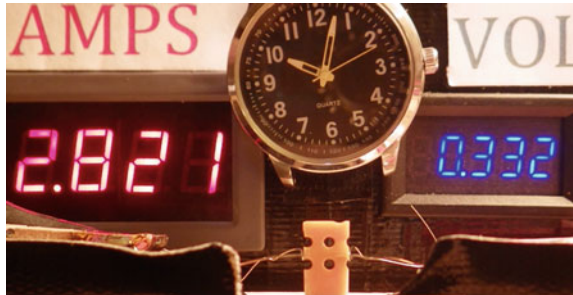
Fig. 14.56 Elapsed time from zero power is 6 s, 0.94 W. No visible smoke or charring (real time captured in video is 10:03:12)
