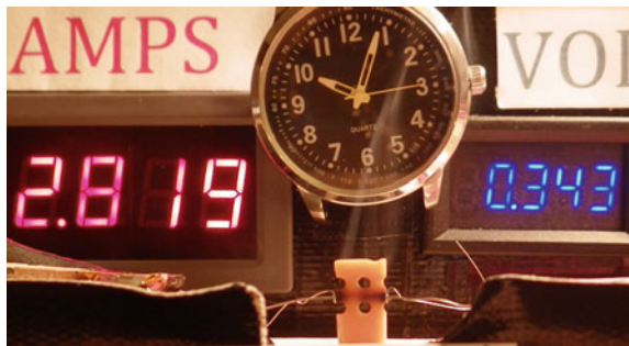
Fig. 14.58 Elapsed time from zero power is 1 min 9 s, 0.97 W. Smoke intensifies with visible charring (real time captured in video is 10:04:15)
