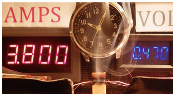
Fig. 14.60 Elapsed time from zero power is 2 min 29 s, 1.8 W. Intense smoke declines (real time captured in video is 10:05:35)
