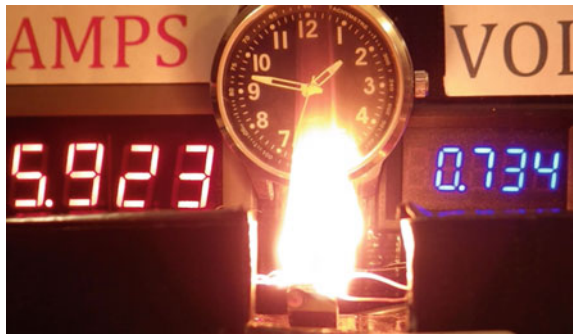
Fig. 14.42 Elapsed time from zero power is 41 s, 4.1 W. Flame peaks (real time captured in video is 01:47:33)
