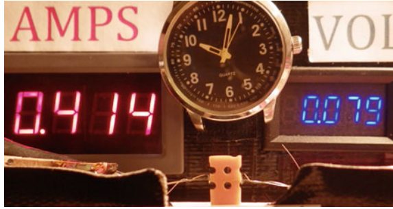
Fig. 14.55 Elapsed time from zero power \sim 1 s, 0.03 W. No visible smoke or charring (real time captured in video is 10:03:06)
