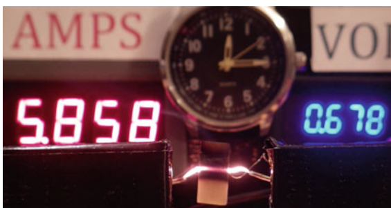
Fig. 14.16 Elapsed time from zero power is 50 s, 3.97 W. Smoke has diminished slightly (real time captured in video is 12:15:10)
