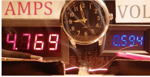
Fig. 14.39 Elapsed time from zero power is 4 min 36 s, 2.83 W. Smoke continues after flame stops (real time captured in video is 08:57:45)
