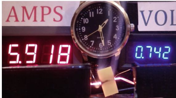
Fig. 14.27 Elapsed time from zero power \sim 1 s, 4.39 W. Smoke with visible charring (real time captured in video is 01:28:40)
