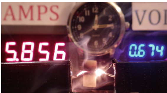
Fig. 14.15 Elapsed time from zero power is 20 s, 3.94 W. Flame with increased charring (real time captured in video is 12:14:40)
