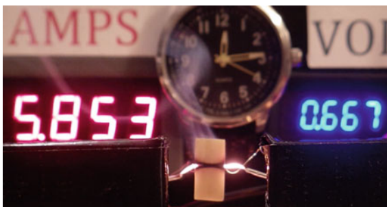
Fig. 14.14 Elapsed time from zero power \sim 1 s, 3.90 W. Smoke with visible charring (real time captured in video is 12:14:20)
