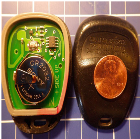
Fig. 6 Contents of the control depicted in Fig. 5 of an electronic control that will lock and unlock a vehicle remotely
