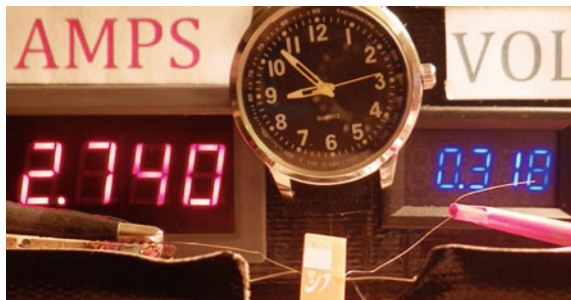
Fig. 14.34 Elapsed time from zero power is 4 s, 1.82 W. No visible smoke or charring (real time captured in video is 08:53:13)
