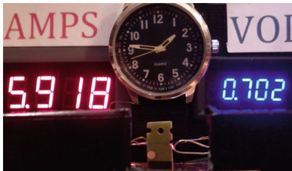
Fig. 14.40 Elapsed time from zero power \sim 1 s, 4.1 W. No visible smoke or charring (real time captured in video is 01:46:42)
