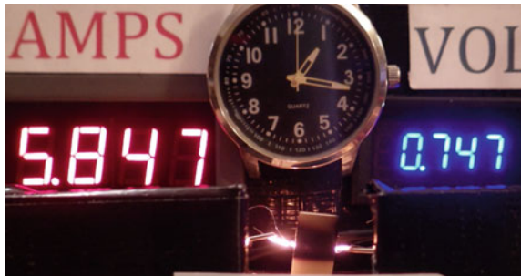
Fig. 14.25 Elapsed time from zero power is 50 s, 4.36 W. Smoke and flame have stopped (real time captured in video is 01:17:00)
