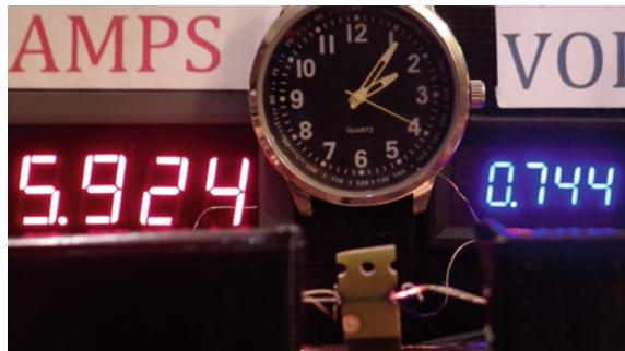
Fig. 14.44 Elapsed time from zero power \sim 1 s, 4.4 W. Charring is instant (real time captured in video is 02:06:20)
