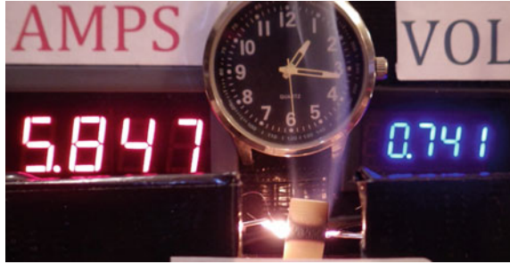
Fig. 14.24 Elapsed time from zero power is 20 s, 4.33 W. Flame extinguishes (real time captured in video is 01:16:29)
