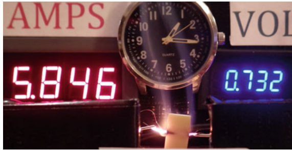
Fig. 14.22 Elapsed time from zero power \sim 1 s, 4.28 W. Smoke with charring at wire entrance and exit locations (real time captured in video is 01:16:10)
