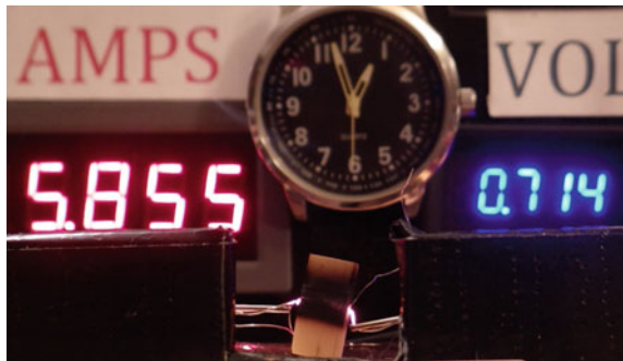
Fig. 14.21 Elapsed time from zero power is 1 min 20 s, 4.18 W. Smoke has stopped (real time captured in video is 12:57:30)
