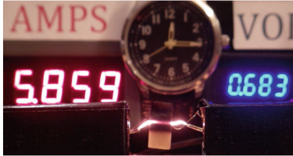
Fig. 14.17 Elapsed time from zero power is 1 min 20 s, 4.00 W. Smoke has stopped (real time captured in video is 12:15:40)
