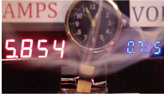
Fig. 14.19 Elapsed time from zero power is 20 s, 4.12 W. Increasing smoke with increased charring (real time captured in video is 12:56:30)
