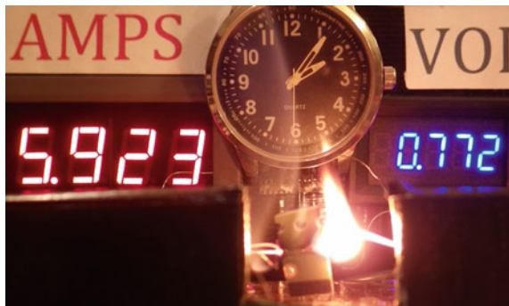
Fig. 14.51 The flame that began in the previous snapshot grew quickly into the flame depicted here over 8 s. Power is 4.5 W at 02:06:30. Elapsed time from zero power is 12 s
