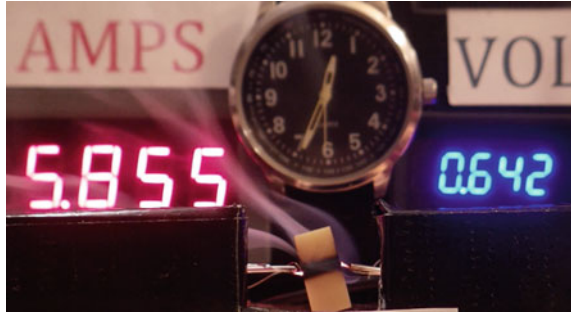
Fig. 14.11 Elapsed time from zero power is 20 s, 3.75 W. Increasing smoke with increased charring (real time captured in video is 12:34:30)
