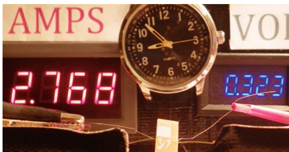
Fig. 14.35 Elapsed time from zero power is 6 s, 0.89 W. No visible smoke or charring (real time captured in video is 08:53:15)
