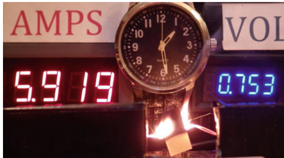
Fig. 14.28 Elapsed time from zero power is 22 s, 4.46 W. Flame (real time captured in video is 01:29:00)
