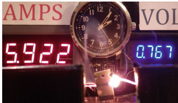
Fig. 14.45 Elapsed time from zero power is 6 s, 4.5 W. Smoke and flame (real time captured in video is 02:06:25)
