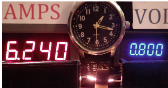
Fig. 14.26 Elapsed time from zero power is 1 min 10 s, 4.99 W. No additional smoke or flame (real time captured in video is 01:17:31)
