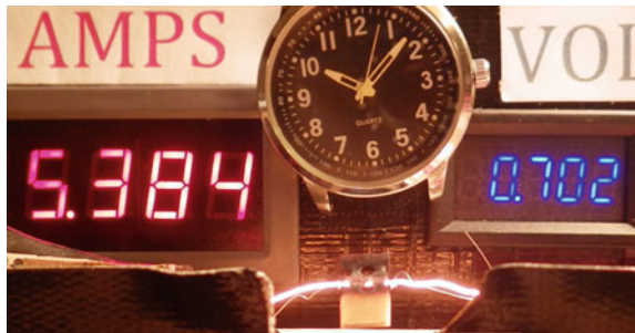
Fig. 14.62 Elapsed time from zero power is 3 min 57 s, Stepped up to 3.8 W (real time captured in video is 10:07:03)
