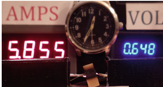
Fig. 14.13 Elapsed time from zero power is 1 min 20 s, 3.79 W. Smoke is no longer visible (real time captured in video is 12:35:30)
