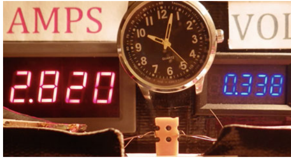
Fig. 14.57 Elapsed time from zero power is 18 s, 0.95 W. Light smoke appears with very light charring (real time captured in video is 10:03:24)
