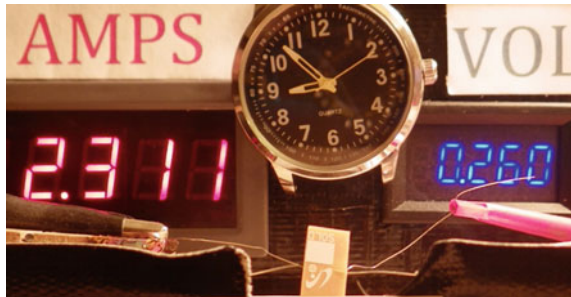
Fig. 14.33 Elapsed time from zero power is 3 s, 0.61 W. No visible smoke or charring (real time captured in video is 08:53:11)
