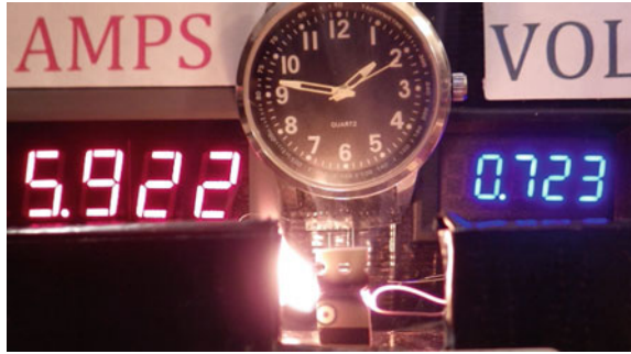
Fig. 14.41 Elapsed time from zero power is 28 s, 4.1 W. Initial flame (real time captured in video is 01:47:10)
