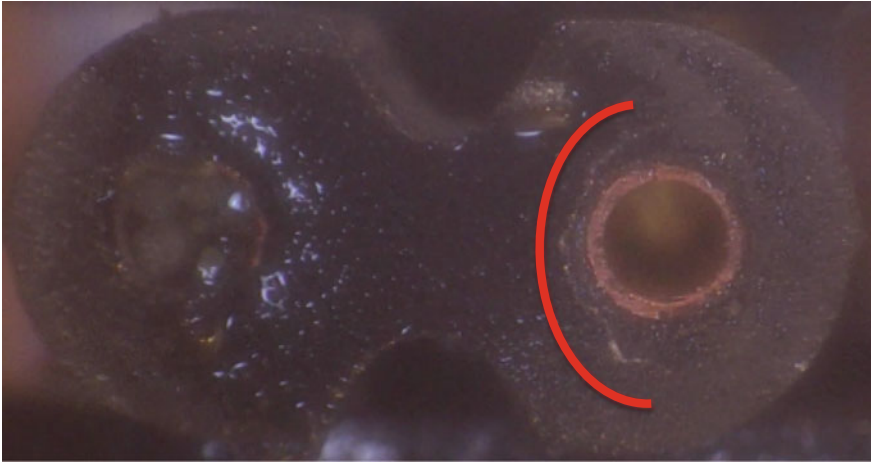
Fig. 7.5 The arc depicted in the previous photo quickly passed current through the liquid to boil it away leaving a new and much wider arc boundary as enclosed by the red curve . (The “jagged marching chain of tiny exploding robots”)
