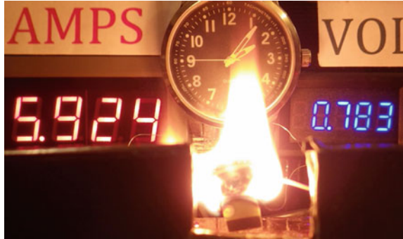
Fig. 14.52 The flame grows continually over 15 s into the flame as depicted to the right. Power is 4.6 W at 02:06:45. Elapsed time from zero power is 15 s
