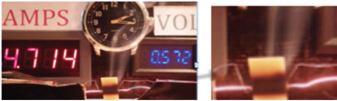
Fig. 14.6 Result of 2.3 W being applied for 1 min after the preceding 1.8 W level (elapsed time from power up is 5 min)
