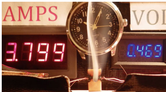
Fig. 14.59 Elapsed time from zero power is 2 min 9 s. Stepped up to 1.8 W. Intense smoke (real time captured in video is 10:05:15)
