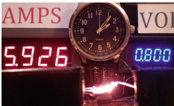
Fig. 14.48 Elapsed time from zero power is 41 s, 4.7 W. Smoke & flame are gone (real time captured in video is 02:07:00)
