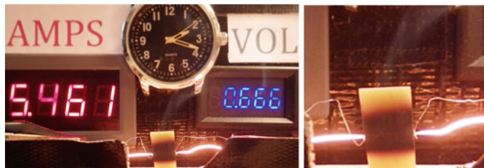
Fig. 14.8 Result of 3.2 W being applied for 1 min after the preceding 2.7 W level (elapsed time from power up is 7 min)
