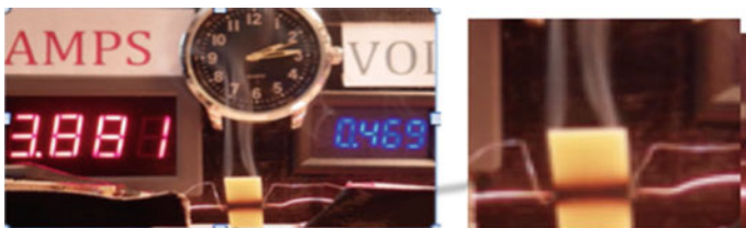
Fig. 14.4 Result of 1.3 W being applied for 1 min after the preceding 0.8 W level for 2 min
