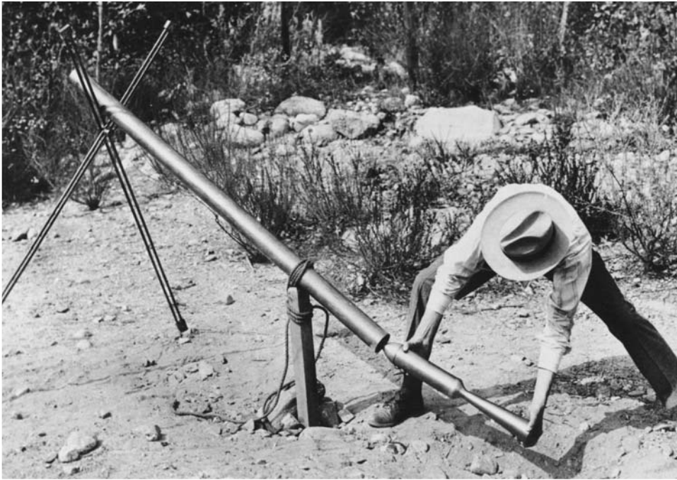
Robert Goddard prepares to test a bazooka-type weapon he developed for the U.S. military in 1918. A small, solid-fuel rocket is inserted in one end of a hollow launching tube. The tube helps aim the rocket toward its target and helps protect the rocketeer launching it from the blast at takeoff.
