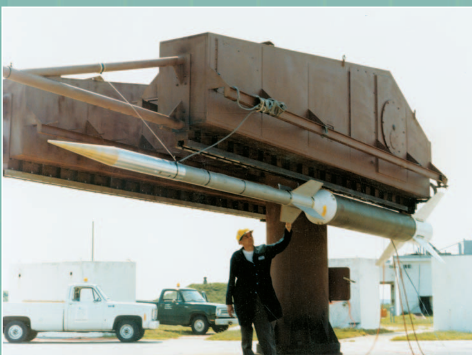
The most popular sounding rocket was the two-stage, solid-propellant Nike-Apache. Large numbers of Nike-Apache rockets were launched by NASA between 1962 and 1980.
