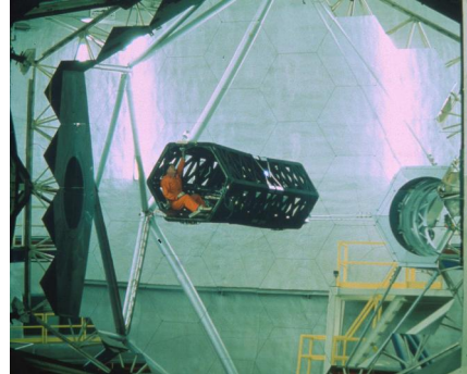
Figure 6. Keck 10-m primary made of 36 segments
