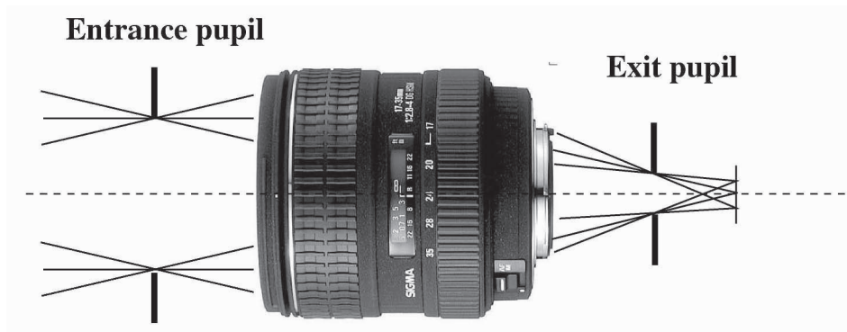
Figure 9. The entrance and exit pupils are the surfaces where the entrance and exit rays coming from the different field positions cross each other. In different terms, the entrance pupil is the aperture 5 of the optical system as seen by an observer located at the position of the object, or at the location of the image for the exit one.
