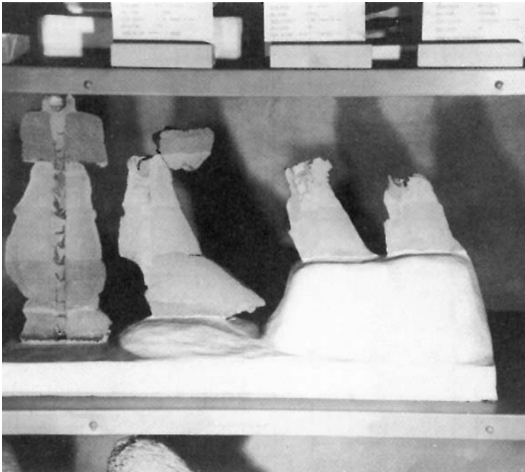
FIGURE 13.29 Photograph of stabilized masses resulting from varying gel times under flowing groundwater.
