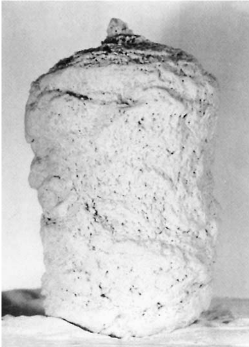
FIGURE 13.9 Uniform stabilization cylinder formed by pulling the pipe shorter distances than in Fig. 13.8 .
