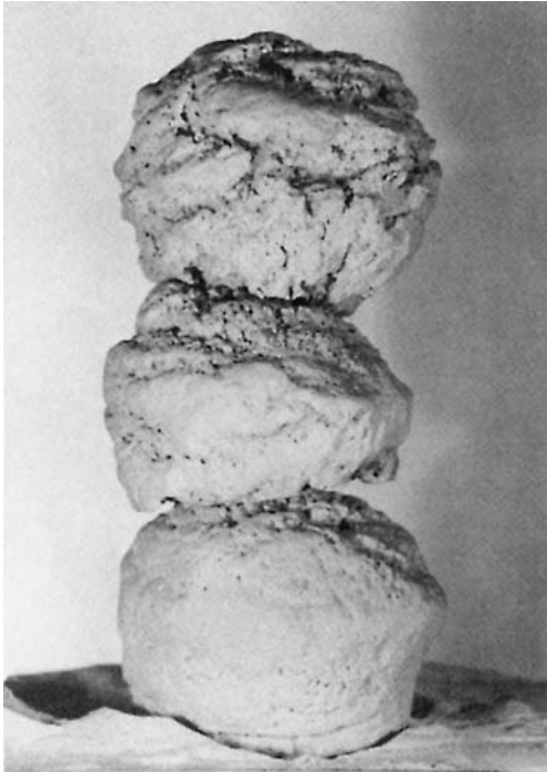
FIGURE 13.8 Tangent stabilized spheres due to excessive distance between injections.
