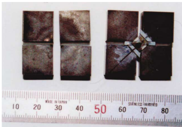
Figure 2. Photos of the Kawai-cell composed of eight SD cubic anvils with an edge length of 14 mm. An octahedral pressure medium of \text{MgO} + 5\% \text{Cr}_2\text{O}_3 and pyrophyllite gasket pieces are placed at the center.
