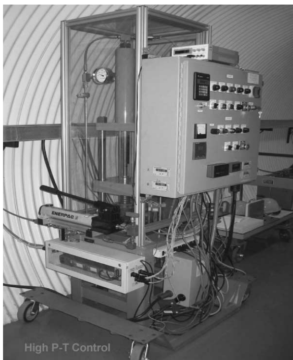
Figure 3. A photograph of the pressure-temperature control system for TAP-98 experiments. This system also includes the displacement (LVDT) meters, the translational stage control, and the remote communication box. This unit is compact and portable and can be used close to and away from neutron flight paths.
