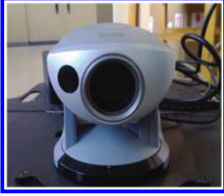
Figure 2. Monocular camera Canon VC-C50i.
