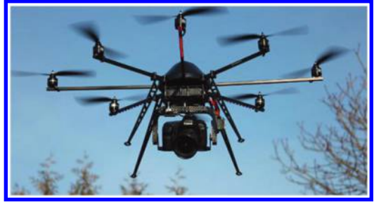
Figure 3. Octo-rotor Aircraft of Draganflyer X8.
