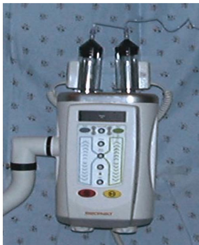
Figure 2.3. Injector set-up for multiphase contrast injection (Medrad, Inc, Indianola, PA). The left syringe is for injection of contrast media, which is followed by saline injection from the right syringe. A Y connector connects both syringes to the patient's intravenous access.
