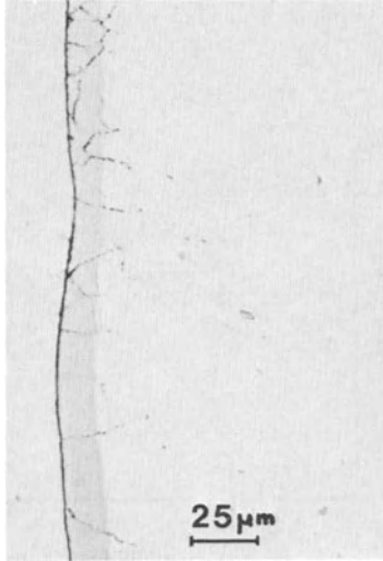
Figure 5 - Nitridation at the surface of a 321 H SS specimen after test in salt containing 1 % \text{BaCl}_2 (775 h, 575°C).
