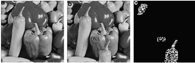
Fig. 8.17 Tamper detection. (a) The watermarked image. (b) Image after attack. (c) The tampered region
