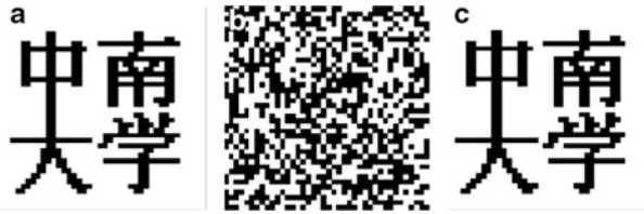
Fig. 8.25 Scrambling effects of the watermark image. (a) The initial image; (b) the scrambled image; (c) the recovered image
