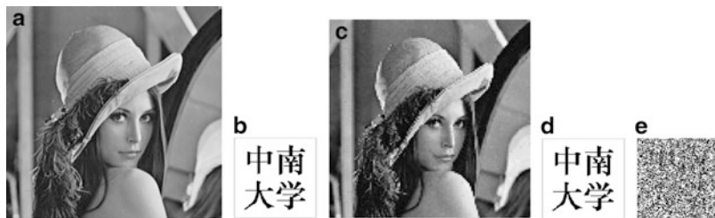
Fig. 8.1 Invisibility and extractability test: (a) Original “Lena” image; (b) Watermark logo; (c) Watermarked image; (d) Extracted watermark with right secret keys. (e) Extracted watermark with wrong key z_0
