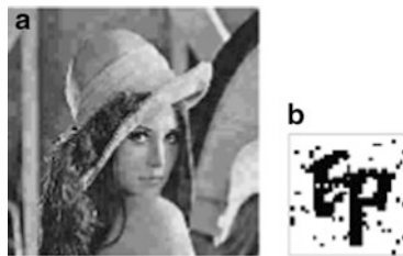
Fig. 8.7 JPEG compression. (a) The watermarked image with JPEG compression quality parameters dropped to 8%; (b) the related watermark extracted from the watermarked image (a)
