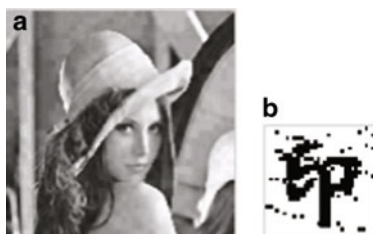
Fig. 8.10 Median filtering. (a) The watermarked image performed one times median filtering operations with window 7 \times 7 ; (b) the related watermark extracted from the watermarked image (a)
