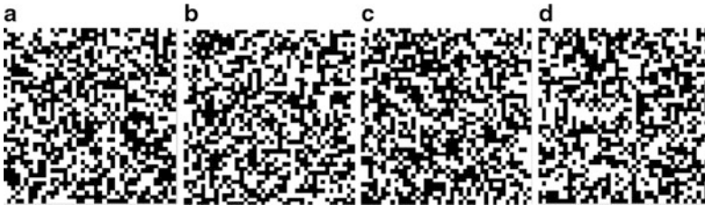
Fig. 8.26 The images of scrambling inverse transformation with wrong keys. (a) key x_0 with error 10^{-16} ; (b) key \alpha with error 10^{-16} ; (c) key \mu with error 10^{-16} ; (d) key m = 10
