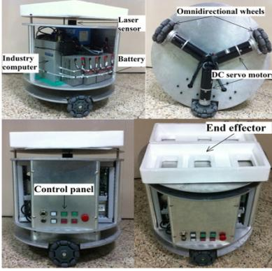
a. Prototype of the experimental OAGV
