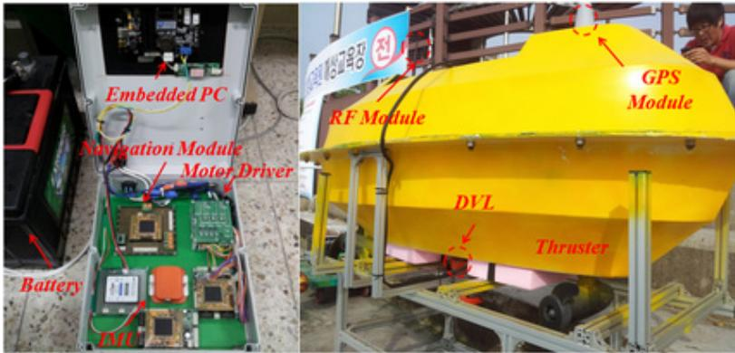
**Fig. 4.** Appearance and components of the USV
