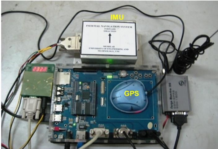
Fig. 5. The hardware configuration of the INS/GPS integrated system
