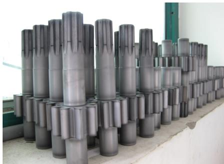
**Fig. 9.** Hydraulic pumping gears
