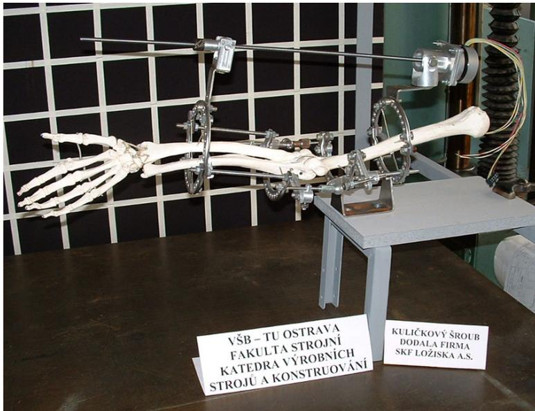
**Fig. 5.** Prototype of the designed external fixator with the stepper motor and movement screw
