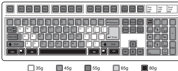
Figure 15.5 Force levels used on KeyTronicEMS keyboards with Ergo Technology.
