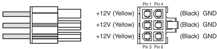
Figure 18.35 PCI Express x16 Graphics 6-pin power connector.
