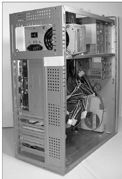
Figure 19.16 Installing the power supply into the chassis.
