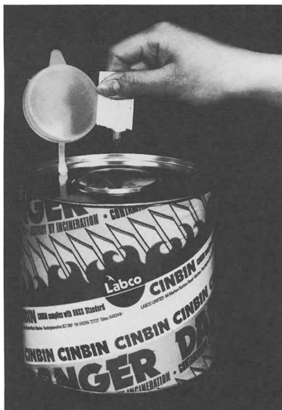
Figure 10.9 Reinforced container for the disposal of sharps
