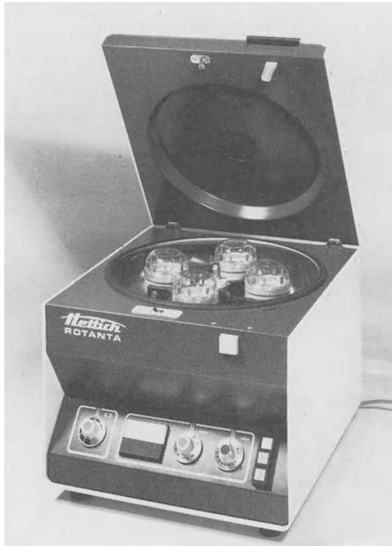
Figure 10.6 Centrifuge fitted with sealed buckets (courtesy A. R. Horwell)
