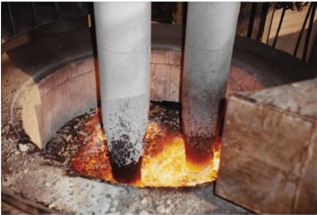
FIGURE 2.5 Picture of the furnace in operation with a charge of SiC and quartz lumps.
