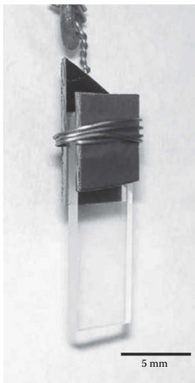
FIGURE 3.23 The 5 mm wide, quartz electrode used in the experiments carried out by Yasuda et al. (Reprinted from Electrochimica Acta , 53, K. Yasuda et al., Direct electrolytic reduction of solid \text{SiO}_2 in molten \text{CaCl}_2 for the production of solar grade silicon, 106–110, Copyright 2007, with permission of Elsevier.)
