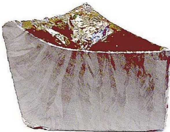
FIGURE 4.10 Section of the first ingot produced by Elkem Solar.
