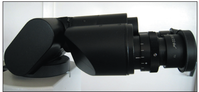
FIGURE 3.10: (A) Tilt-head binocular focusable wide-angle oculars with the tilt-head tilted up. (B) Tilt-head tilted down to accommodate a shorter-stature surgeon-pathologist.
