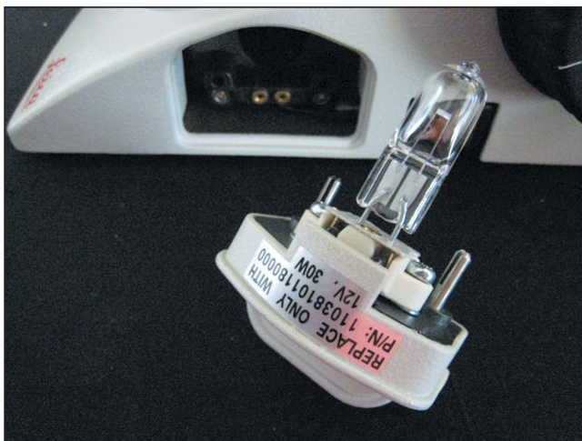
FIGURE 3.7: Halogen substage lighting. Having a spare bulb available is essential.
