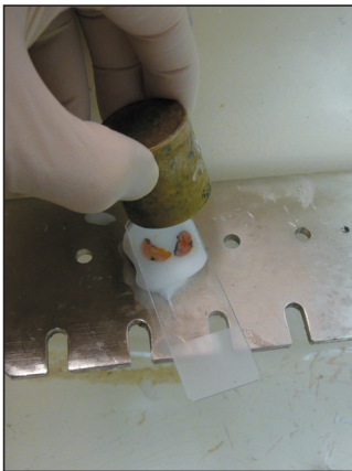
FIGURE 6.25: Specimen/chuck being frozen as one contiguous block.
