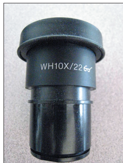
FIGURE 3.2: Wide-angle, high-quality focusable ocular lens.
