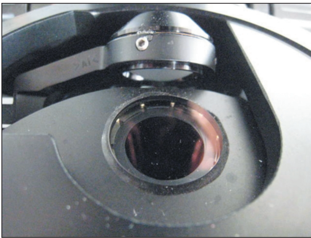
FIGURE 3.12: (A) Condenser with leaves closed down. (B) Condenser leaves are wide open.
