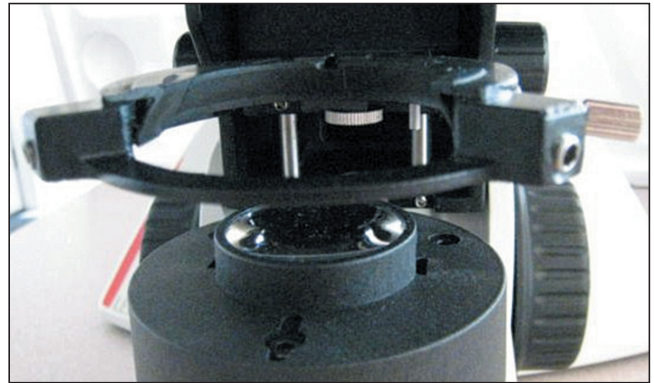
FIGURE 3.14: If the 10-sided figure is not centered in your field of vision, center it using the two centering screws on the condenser. The actual adjustment screws are not in place in this photo but lie at the ends of the two rectangular blocks in the ring that holds the condenser. The third screw on the condenser (silver screw on the right side of the photo) is used only to secure the condenser in its mount, and almost never needs to be touched.
