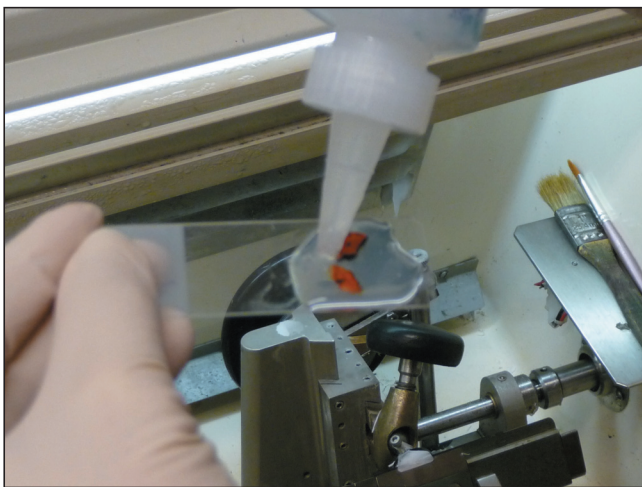
FIGURE 6.21: Bisected specimen on mounting slide covered with tissue freezing medium.
