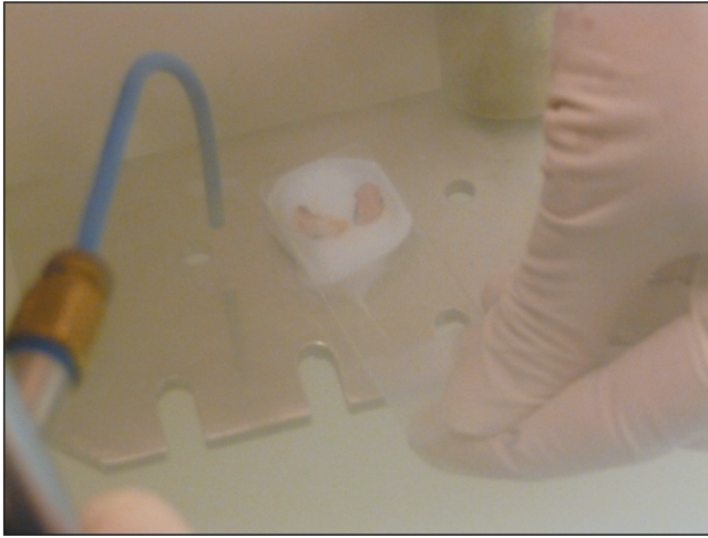
FIGURE 6.24: Specimen/chuck being frozen as one contiguous block.
