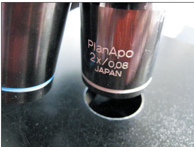
FIGURE 3.4: 2x lens. Using a 1\times – 2.5\times lens for low-power viewing is essential for efficient Mohs surgery.
