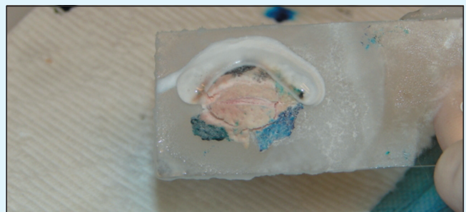
FIGURE B.8: To further aid the edges in adhering to the slide, add dabs of optimal cutting temperature medium as needed.
