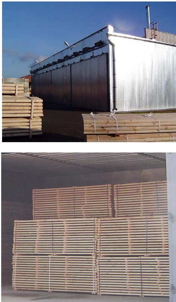
Figure 1.1. Block of four conventional kilns with a load volume of 50 m 3 of timber each (a). Formation of stacks inside the chamber (b). Klichev Forestry, Belarus.
