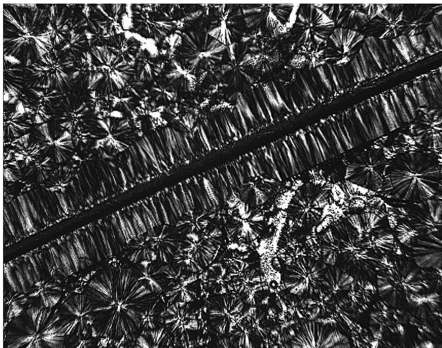
Figure 12. Microphotograph obtained by polarized light microscopy of an iPP/Sisal fibre system crystallized by cooling from the melt at 210 °C. Cooling rate = 5 °C/min.
