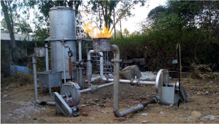
Figure 11. Open core down draft gasifier.
