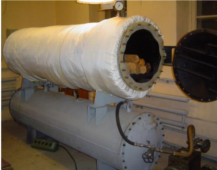
Figure 1.11. Photo of the experimental vacuum-convective drying kiln.
