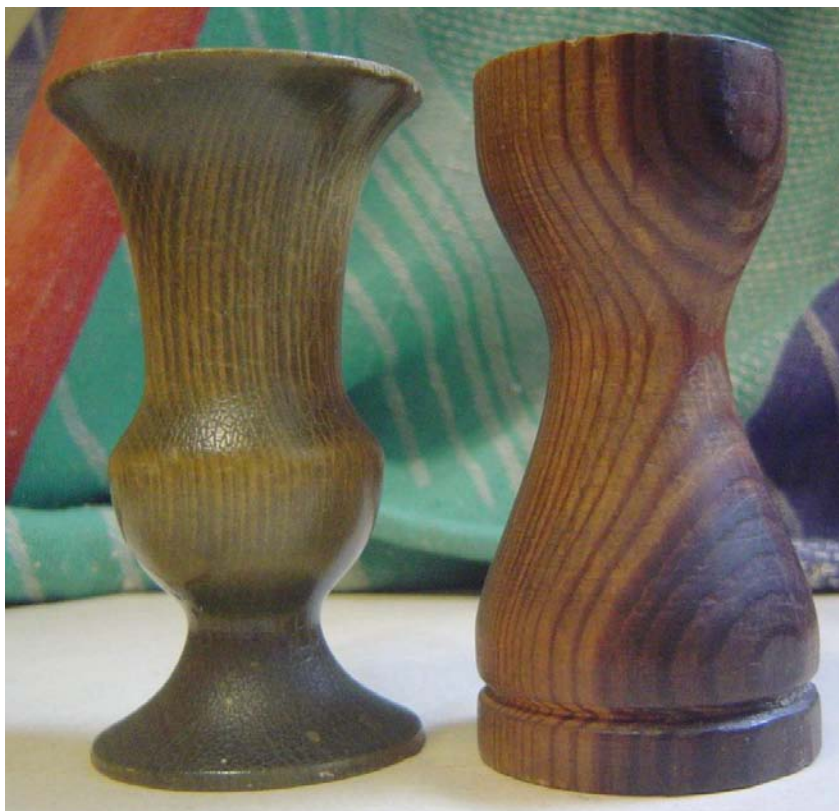
Figure 2.2. Samples of products carved of impregnated birch (left) wood and pine (right) wood.
