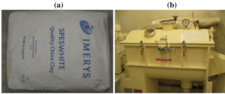
Plate 6.11 a Speswhite China clay. b Mixer for preparation of clay slurry
