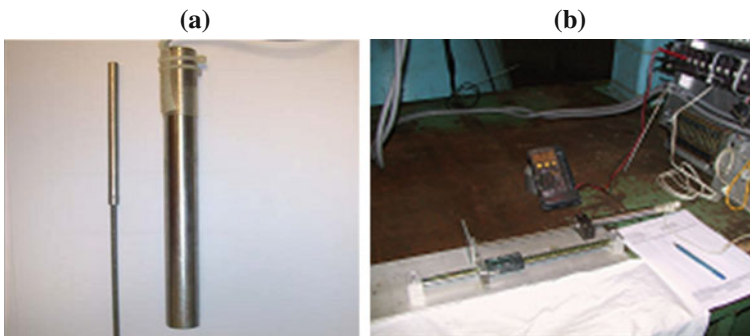
Plate 6.20 a Linear variable differential transformer (LVDT). b Calibration of LVDT
