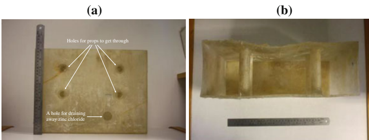
Plate 6.4 A manufactured rubber bag. a Elevation view. b Plan view
