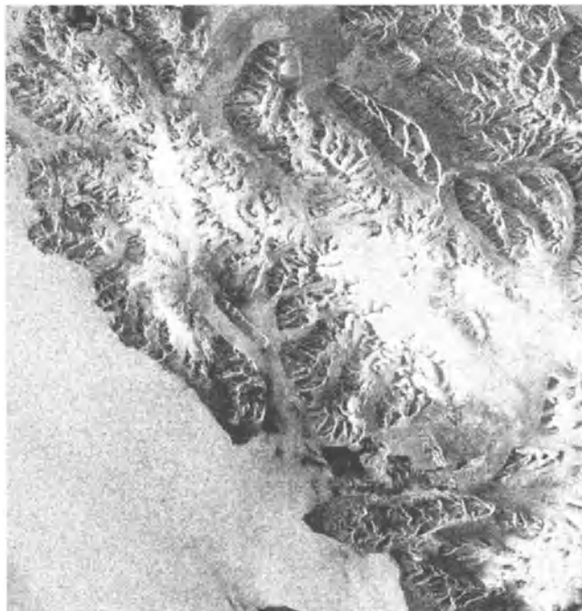
Figure 3. ERS-1 (C-VV) SAR image of northwestern Spitsbergen showing the effects of surface and subsurface properties as well as topography on the resulting radar return.
