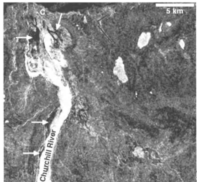
Figure 3. SAR subsense of the lowermost reaches of the Churchill River, Manitoba, 13 April 1998. The four white arrows indicate river ice that is frozen to the bottom. The very bright features in the upper right quadrant are ice-covered shallow lakes. Churchill (C) is located at 58.72°N, 94.12°W. North is at the top of the frame. The original ERS-2 image (©ESA) was radiometrically corrected then filtered to reduce speckle by C. R. Duguay, who provided the subsense.
