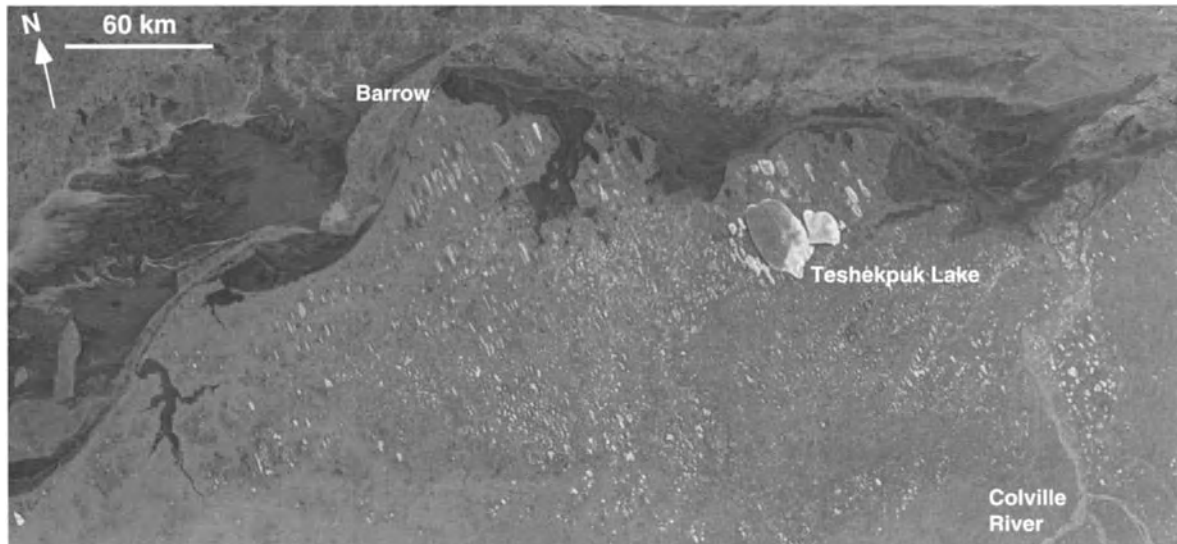
Figure 8. SAR image subscene of the western region of the North Slope of Alaska, 12 May 1997. Barrow is located at 71.30°N, 156.82°W. The many small bright features are areas of floating lake ice. The length of the bottom of the image is equivalent to 480 km on the ground. The original RADARSAT-1 ScanSAR Wide B image (©CSA) is from ASF.
