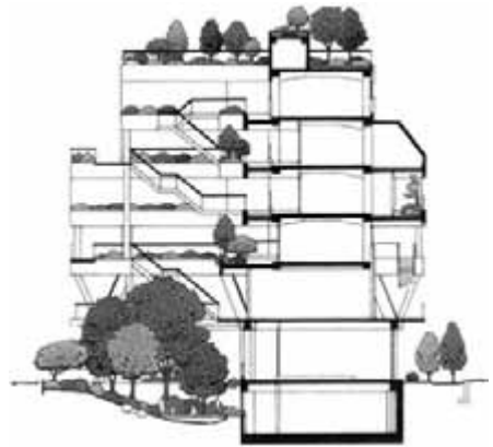
Fig. 4.86 Building section showing urban natural habitats. Drawing courtesy of Shu-Koh-Sha Architecture and Urban Design Studio.
