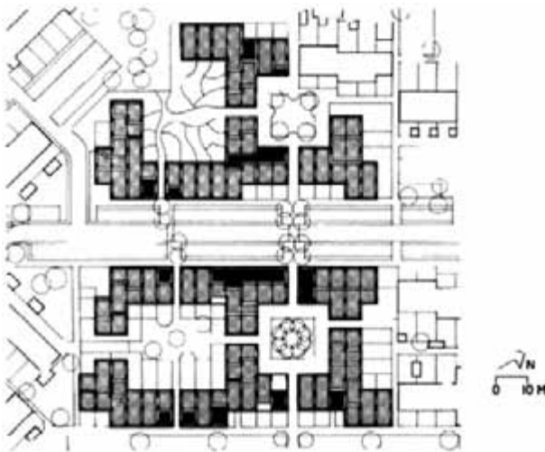
Fig. 4.31 Site plan showing courtyards, parking and non-residential uses. Drawing courtesy of Frans van der Werf.
