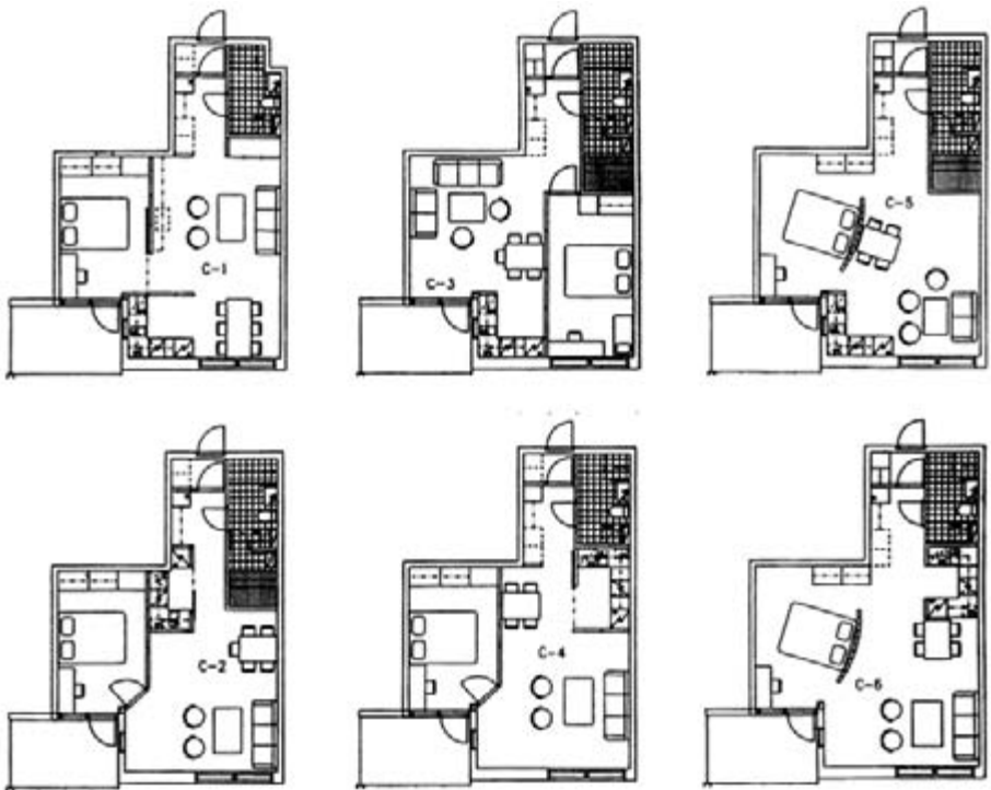
Fig. 4.100 Optional dwelling unit plans. Drawing courtesy of Architecture Office Kahri and Co.
