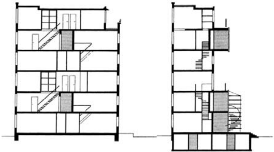
Fig. 4.96 Building cross-sections showing corridors on alternating floors. Drawing courtesy of De Jager & Lette Architects.
