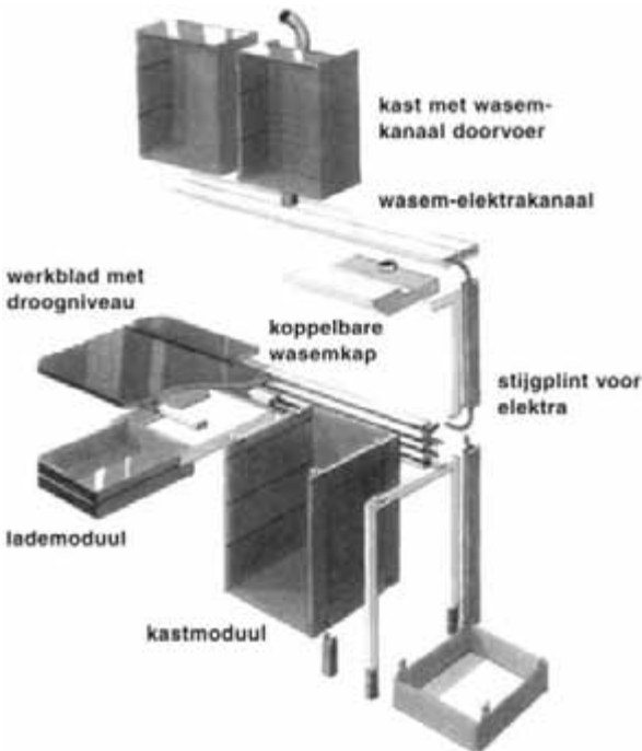
Fig. 7.6 Plug-and-play kitchen. Drawing courtesy of Esprit.
