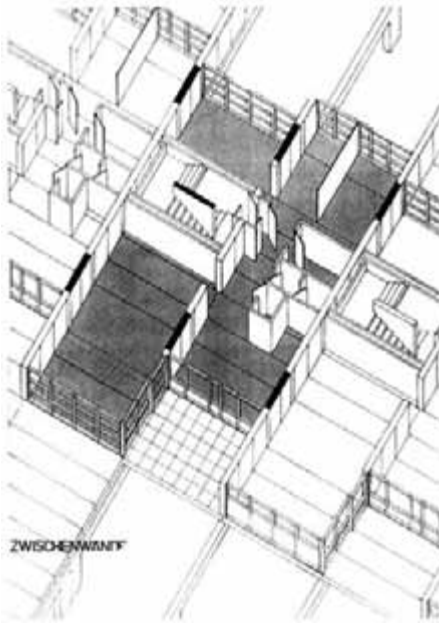
Fig. 4.14 Schematic drawing of the Support parcellation (subdivision). Drawing courtesy of the Office of Architect Professor Ottokar Uhl.
