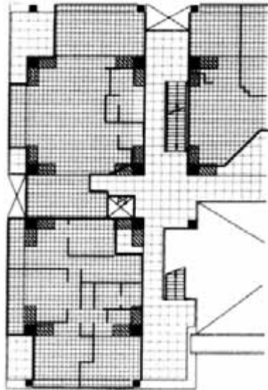
Fig. 4.87 Modular grids for coordination. Drawings courtesy of Seiichi Fukao.
